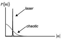
FIG. 7. The quasiprobability function  $P(|\alpha|)$  for a chaotic excitation is Gaussian in form, while for a stable laser beam it takes on nonzero values only near a fixed value of  $|\alpha|$ .
