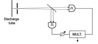
FIG. 3. The Hanbury Brown–Twiss photon correlation experiment. Light from an extremely monochromatic discharge tube falls on a half-silvered mirror which sends the split beam to two separate photodetectors. The random photocurrents from the two detectors are multiplied together and then averaged. The variable time delay indicated is actually achieved by varying the distance of the detector  $D_2$  from the mirror.
