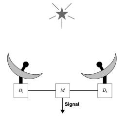
FIG. 2. The intensity interferometry scheme of Hanbury Brown and Twiss. Radio-frequency waves are received and detected at two antennas. The filtered low-frequency signals that result are sent to a device that furnishes an output proportional to their product.
