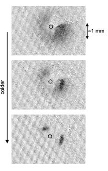
FIG. 5. Time-of-flight absorption images of some of the first condensates produced at MIT in the night of September 29, 1995. After the magnetic quadrupole trap was switched off, the atom cloud expanded ballistically. However, since the optical plug (indicated by black circles) could not be turned off at the same time, it distorted the expanding cloud. Still, as the temperature was lowered from top to bottom, a distinctly sharp shadow appeared marking the presence of a condensate.
