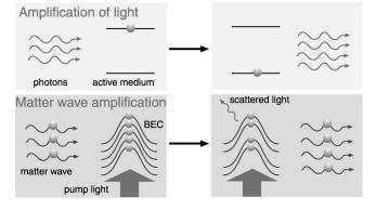
FIG. 17. Amplification of light and atoms: In the optical laser, light is amplified by passing it through an excited inverted medium. In the MIT atom amplifier, an input matter wave is sent through a Bose-Einstein condensate illuminated by laser light. Bosonic stimulation by the input atoms causes light to be scattered by the condensate exactly at the angle at which a recoiling condensate atom joins the input matter wave and augments it.
