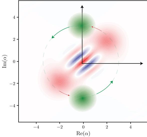
FIG. 4. Wigner function of the state of a cat qubit during the execution of an  $X$  operation. The green dots are the Wigner functions of the instantaneous steady states of the dynamics  $\dot{\rho} = \kappa_2 \mathcal{D}[\hat{a}^2 - \alpha(t)^2]$ . These attractive points are slowly rotated from  $\pm\alpha$  to  $\mp\alpha$  on the dashed circle, as shown by the green arrows. When this rotation is performed slowly, the cat follows the attractors (red arrows).
