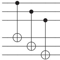
FIG. 7. Transversal implementation of the logical CNOT. For clarity, the number of cat qubits per repetition cat qubit is  $n = 3$ . Here, the three upper lines represent the control repetition cat qubit, and the three bottom ones represent the target one.
