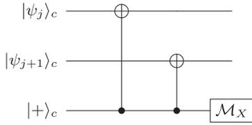
FIG. 5. Joint-parity measurement between two neighboring cat qubits  $j$  and  $j + 1$  of a repetition cat qubit, using one ancilla cat qubit. Note that the error propagation from ancilla cat qubit to data ones is exponentially suppressed by the cat size.
