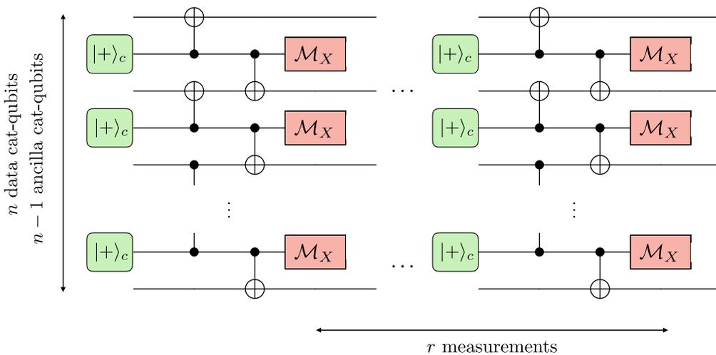
FIG. 6. Quantum error correction circuit for a repetition cat qubit. One repetition cat qubit, composed of data cat qubits and ancilla cat qubits (in green), is protected from errors by performing  $r$  rounds of error detection.
