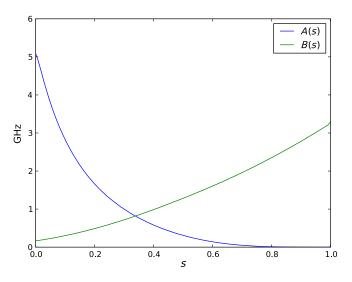
FIG. 8. Quantum annealing schedules employed by the D-Wave processor, where  $s = t/t_f$ .
