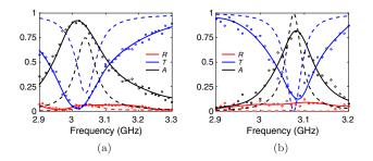
FIG. 10. Measured and the corresponding simulated reflection, transmission, and absorption coefficients for the fabricated metasurfaces with (a) single- and (b) double-turn helical inclusions. The dots denote measured values. The solid lines are the envelope curves of the measured data. The dashed lines show the corresponding simulated coefficients of the measured samples.
