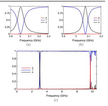
FIG. 6. Simulated power reflection R, transmission T, and absorption A coefficients for infinite arrays of (a) single- and (b) double-turn helical inclusions. (c) Response of the double-turn helix array in a wide frequency range.
