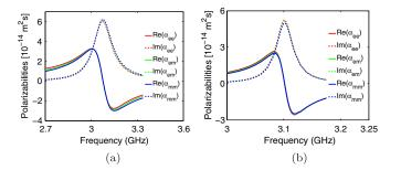
FIG. 5. Individual normalized polarizabilities of the designed (a) single- and (b) double-turn helical inclusions.
