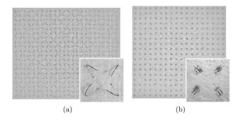
FIG. 9. Fabricated metasurfaces of (a) single-turn and (b) double-turn helices comprising, respectively, 480 and 324 elements embedded in plastic foam.
