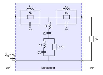
FIG. 7. An equivalent circuit of the proposed absorbers matched at all frequencies. The resistive load  $\eta_0 = 377 \ \Omega$  denotes the impedance of free space behind the absorber.
