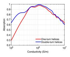
FIG. 4. Absorption coefficient versus conductivity of the inclusion material at the operating frequency of 3 GHz.
