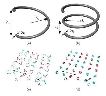
FIG. 3. (a) Single-turn and (b) double-turn helical inclusions. (c) Arrangement of the single-turn and (d) double-turn helical inclusions in the arrays. Blue and red colors denote right- and left-handed helices, respectively.
