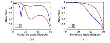
FIG. 8. The absorption level A = 1 - R - T in a metasurface with (a) single-turn and (b) double-turn helical elements versus the incident angle.
