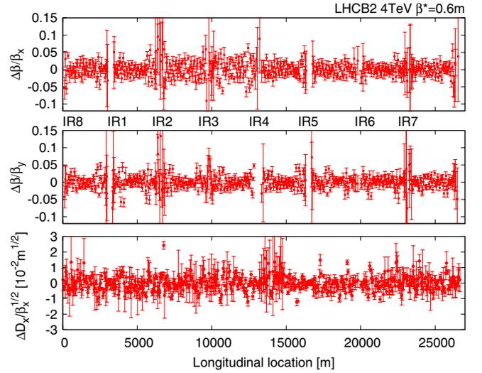
FIG. 8. Beam 2  $\beta$  beating and normalized dispersion beating after global correction at  $\beta^* = 0.6$  m.
