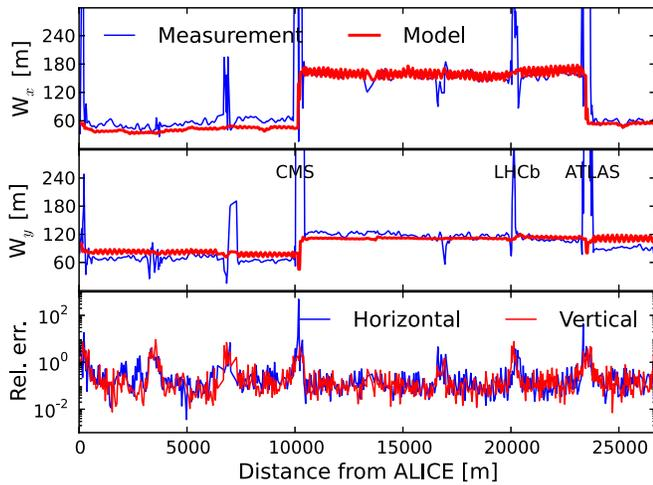
FIG. 12. Beam 1 horizontal (upper) and vertical (middle) Montague functions as defined in Eq. (3). The model function is shown in red, and the measurement in blue. The relative error of the measurements is shown in the lower plot. The figure shows the case for 0.6 m  $\beta^*$  optics at 4 TeV beam energy, after corrections.
