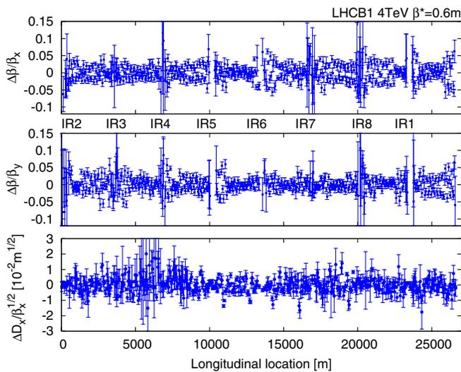
FIG. 7. Beam 1  $\beta$  beating and normalized dispersion beating after global correction at  $\beta^* = 0.6$  m.
