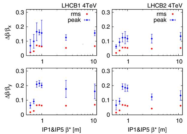
FIG. 9.  $\beta$  beating after global correction for  $\beta^* \leq 0.7$  m and after local correction for  $\beta^* \geq 0.8$  m. Beam 1 (left) and beam 2 (right), horizontal (top) and vertical (bottom) plots showing the peak and rms  $\beta$ -beating values versus  $\beta^*$ .
