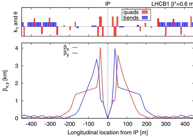
FIG. 1. Layout of the main interaction region (top) and  $\beta$  functions (bottom) versus longitudinal location from the IP for  $\beta^* = 0.6$  m.
