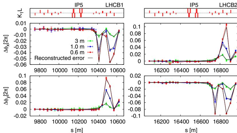
FIG. 6. Illustration of the segment-by-segment technique applied to IR5 simultaneously to the two beams and three different  $\beta^*$ . The black lines show the reconstructed error model.
