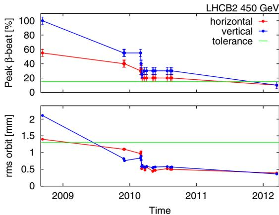
FIG. 2. Measured peak  $\beta$  beating (top) and rms orbit (bottom) at injection for beam 2 versus time.
