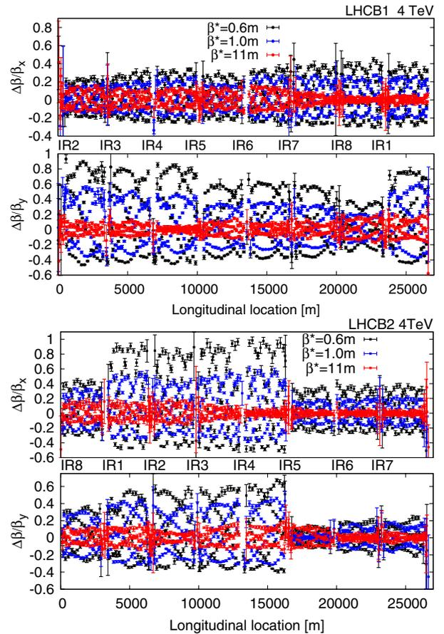
FIG. 3. Beam 1 (top) and beam 2 (bottom)  $\beta$  beating at three IP1 and IP5  $\beta^*$  values during the squeeze of the virgin machine.
