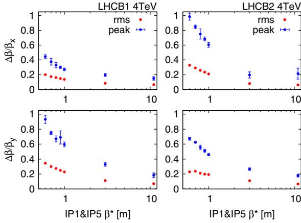
FIG. 4.  $\beta$  beating of the virgin machine along the squeeze. Beam 1 (left) and beam 2 (right), horizontal (top) and vertical (bottom) plots showing the peak and rms  $\beta$ -beating values versus  $\beta^*$ .
