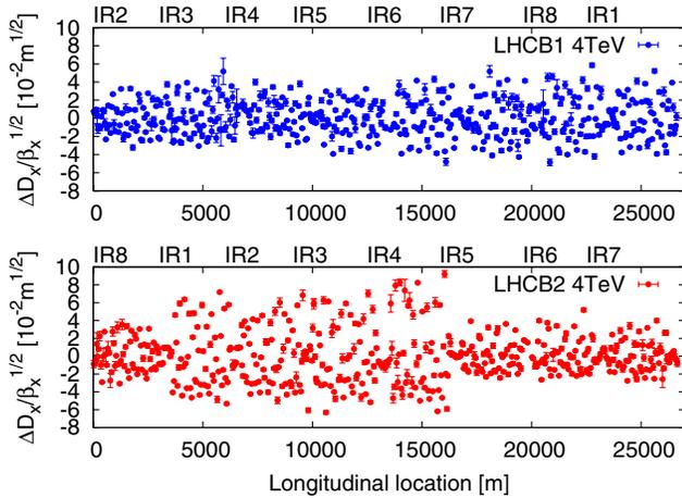
FIG. 5. Normalized dispersion beating for beam 1 (top) and beam 2 (bottom) for the virgin machine at  $\beta^* = 0.6$  m.
