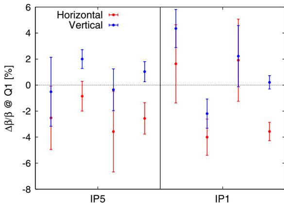
FIG. 10.  $\beta$  beating from  $K$  modulation at the first quadrupoles by IP1 and IP5.
