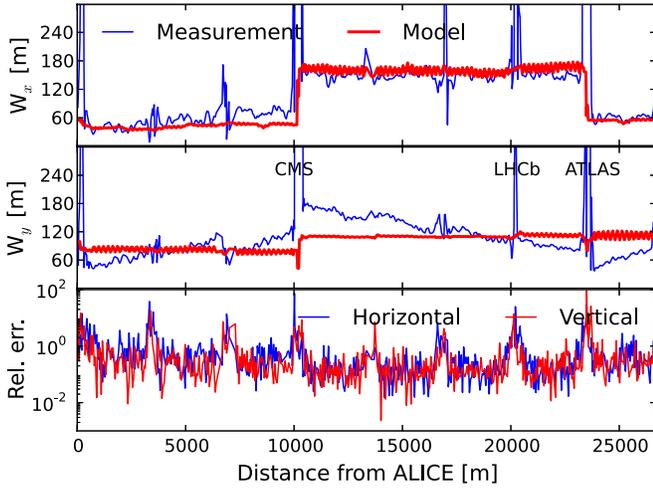
FIG. 11. Beam 1 horizontal (upper) and vertical (middle) Montague functions as defined in Eq. (3). The model function is shown in red, and the measurement in blue. The relative error of the measurements is shown in the lower plot. The figure shows the case for 0.6 m  $\beta^*$  optics at 4 TeV beam energy, before corrections.
