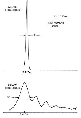
FIG. 2. Emission spectrum of the laser oscillator above threshold (top) and of the spontaneous radiation emitted by the electron beam (bottom).
