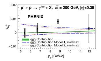
FIG. 2. Transverse single-spin asymmetry of isolated direct photons measured at midrapidity  $|\eta| < 0.35$  in  $p^{\uparrow} + p$  collisions at  $\sqrt{s} = 200$  GeV. An additional scale uncertainty of 3.4% due to the polarization uncertainty is not shown.
