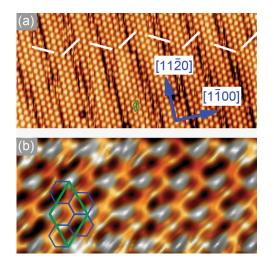
FIG. 1 (color). STM images of the  $(2 \times 2)$ -reconstructed ZrB<sub>2</sub>(0001) surface with different length scales: (a) 20 nm× 9.5 nm, I = 55 pA,  $V_s = 700$  mV, (b) 4.2 nm × 2 nm, I = 600 pA,  $V_s = 100$  mV. The white lines emphasize the direction of offsets between successive domains. The  $(2 \times 2)$  UC and the honeycomb mesh are emphasized by green and blue solid lines, respectively.
