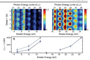
FIG. 2 (color). Energy spectra as a function of delay from electrons liberated from the 3s shell (a) and the 3p shell (b), respectively. (c) Retrieved delays corrected for the Cr group delay. Also shown are the 3p delays shifted down in energy for comparison with the 3s delays (dashed line).
