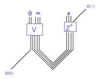
FIG. 5. A circuit for teleporting a single qubit through an entangled state of N + N qubits. At this stage the unitary operator Z on Bob's side is unspecified.
