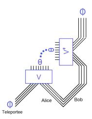
FIG. 22. Circuit diagram for large-system teleportation.
