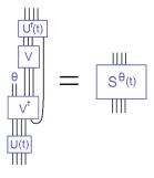
FIG. 10. Definition of the N qubit unitary operator  $S^{\theta}(t)$ . One of the qubits on the right side loops from the bottom of  $V^{\dagger}$  to the bottom of  $U^{\dagger}(t)$ . We'll call it the "looping qubit".
