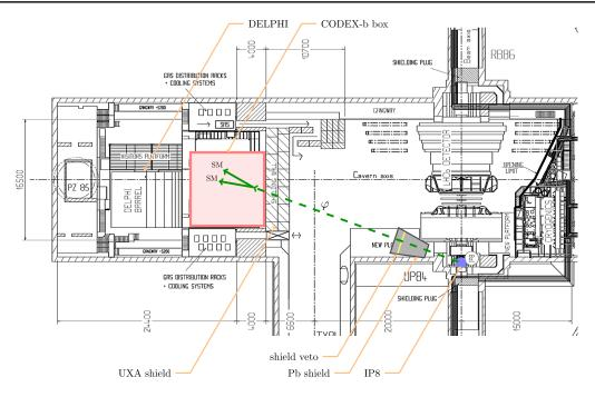
FIG. 1. Layout of the LHCb experimental cavern UX85 at point 8 of the LHC [66], overlaid with the CODEX-b apparatus.
