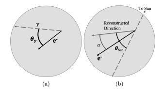
FIG. 2. Definitions of angles referenced in this paper:  $\theta_{\gamma}$  is the angle between the electron's travel direction and the photon direction;  $\alpha$  is the angle between the true and reconstructed direction of the electron; and  $\theta_{\text{Sun}}$  is the angle between the reconstructed event direction and the solar direction (assumed true direction of the neutrino).
