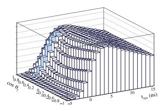
FIG. 3. Distribution of photon hits in  $\cos \theta_{\gamma}$  and  $t_{\rm res}$  for simulated 6 MeV electrons in LAB with a PPO concentration of 0.6 g/L. A clear peak can be seen at low  $t_{\rm res}$  near the expected Cherenkov angle,  $\cos \theta_{\gamma} = 0.66$ , highlighted in blue.
