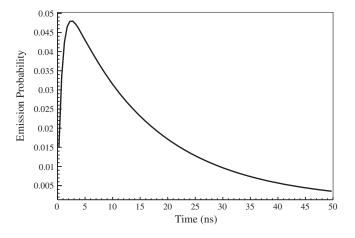
FIG. 1. Parametrized time profile of scintillation light emission for electrons in LAB with 0.6 g/L PPO based on comparisons of <sup>214</sup>Bi background events in data and simulations.
