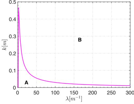
FIG. 1. Plot of the work  $W$  for  $k$  and  $\lambda$ . Areas A and B represent  $W \geq 2mc^2$  and  $W < 2mc^2$ , respectively. The magenta line denotes  $W = 2mc^2$ .
