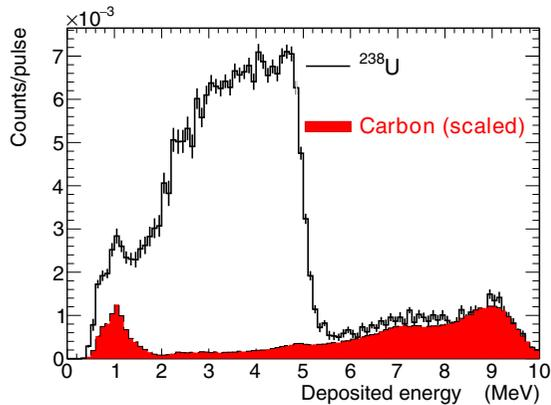
FIG. 2. Carbon and  $^{238}\text{U}$  deposited energy spectra, per histogram bin, for  $m_{\text{cr}} > 1$  and with the sample-out and beam-off backgrounds subtracted, where the carbon spectrum has been scaled above 7 MeV to match the number of  $^{238}\text{U}$  counts to allow an estimation of the scattering contribution to the  $^{238}\text{U}$  data.
