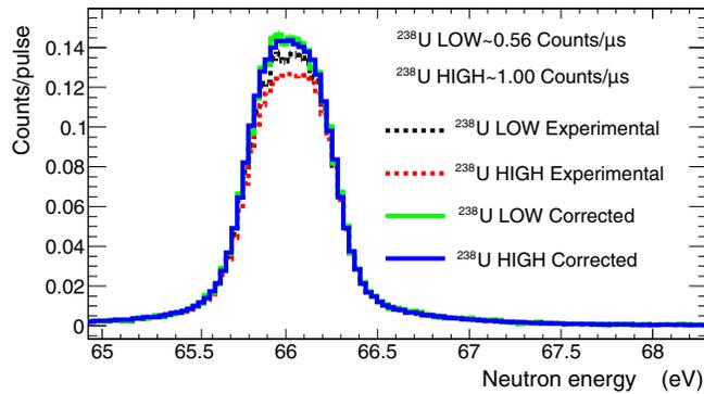
FIG. 4. The highest count rate in the data is found in the resonance at 66 eV. The asymmetrical resonance shape in the  $1.0 \times 10^{12}$  ppp (HIGH) data is removed after correcting for pileup and dead-time.
