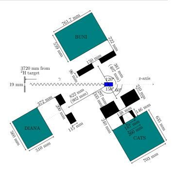
FIG. 1. A schematic plan view of the experimental setup. Gray: beam collimator; wavy line: photon beam; blue box: deuterium target; black regions: detector front and inner collimators; green boxes: scintillators (NaI(Tl) and plastics). The distances between the target and the detectors were different in 2011 and 2015. The 2011 values are indicated in brackets.
