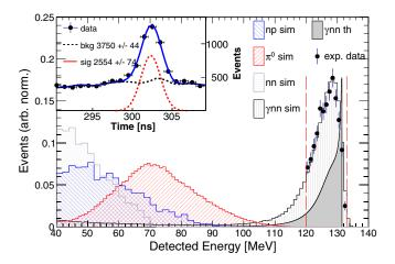
FIG. 3. Simulated energy spectra of dominant reaction channels alongside the measured energy spectrum and a theoretical energy spectrum of  $\pi^-$  RC. Inset: A typical fit to a timing-coincidence spectrum for events inside the cut  $E_{\text{det}} \in [120, 133]$  MeV for yield determination.
