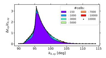
FIG. 5. Rms emittance growth versus  $k_{0xy}$  for self-consistent 2D PIC simulation and different total numbers of FODO cells.
