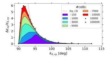
FIG. 6. Rms emittance growth versus  $k_{0xy}$  for self-consistent 3D PIC simulation and different total numbers of FODO cells.
