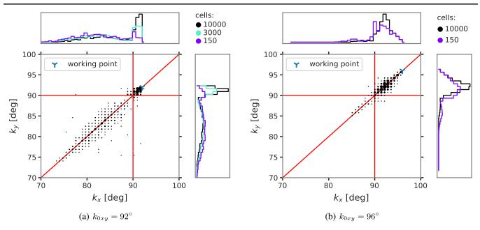
FIG. 7. Tune footprints in halo and outer core region for 3D PIC simulation.
