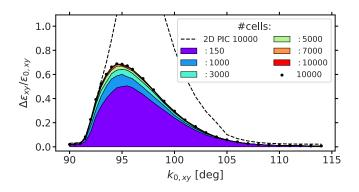
FIG. 8. Rms emittance growth versus  $k_{0xy}$  for different total numbers of FODO cells and 2D FSM computation, with the 2D PIC result in dashed for comparison.
