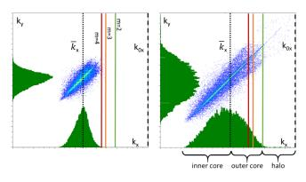
FIG. 3. Spectral distributions  $f_0(k_{xy})$  (as unnormalized intensity (per bin of  $k_{xy}$ ) for 2D waterbag (lhs) and Gaussian (rhs) distributions generated for a fixed  $k_{0xy}$ . Also shown are locations of  $\bar{k}_x$  and of the m = 2, 3, 4 coherent mode lines (i.e., mode frequencies divided by m).
