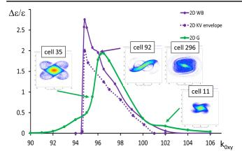
FIG. 1. Rms emittance growth versus  $k_{0xy}$  for the stopband above 90° for 2D waterbag and Gaussian distributions after 300 FODO cells. Inserts showing x - x' phase space at different  $k_{0xy}$  and cells.
