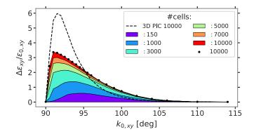
FIG. 9. Rms emittance growth versus  $k_{0xy}$  for different total numbers of FODO cells and 3D FSM computation, with the 3D PIC result in dashed for comparison.
