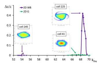
FIG. 2. Rms emittance growth versus  $k_{0xy}$  for the stopbands above 60° and 45° for 2D waterbag and Gaussian distributions after 300 FODO cells. Inserts showing x - x' phase space at different  $k_{0xy}$  and cells.
