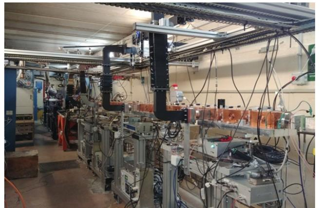
FIG. 9. TOP-IMPLART 35 MeV segment currently in operation.
