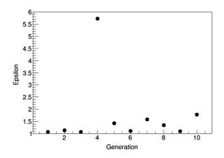
FIG. 10. The *epsilon* test of convergence in our online study:  $\epsilon$  is the scale factor such that the *i*th generation frontier set  $X_i$  dominates the rescaled frontier set  $\epsilon X_{i+1}$ . The algorithm converges as  $\epsilon$  approaches unity. The figure shows that the algorithm is still providing improvement at the end of the allotted time. Comparison with Fig. 9 shows that this improvement is mainly due to reduction in the orbit error.
