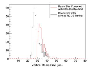
FIG. 6. Histogram of hundreds of experimental vertical beam size measurements both after applying just the standard Levenberg-Marquardt minimization of dispersion and coupling and after additional tuning with the RCDS algorithm using the best 8 eigenparameters. A modest but unambiguous improvement is observed. Note also the high-side tails of the measurement distributions.
