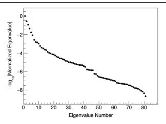
FIG. 1. The spectrum of eigenvalues obtained from the Hessian matrix of the emittance, normalized so that the first eigenvalue is equal to one. Note the logarithmic vertical scale. The Hessian matrix and its spectrum are available as Supplementary Material [27].
