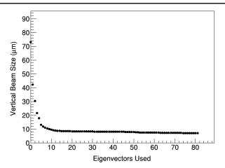
FIG. 3. The average simulated beam size over 1000 instances of a lattice with random misalignments after minimizing the beam size using our first N eigenparameters. The average initial beam size is shown by the point lying on the vertical axis. Note the rapid decrease in beam size from the first few eigenparameters.
