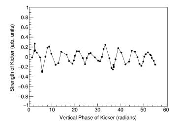
FIG. 2. The relative strengths of the kickers used in the first eigenvector as a function of their vertical betatron phase in CESR. Their arrangement in the shape of a betatron wave is readily apparent. The vertical tune is 8.79, nearly matching the 9 crests of the wave.
