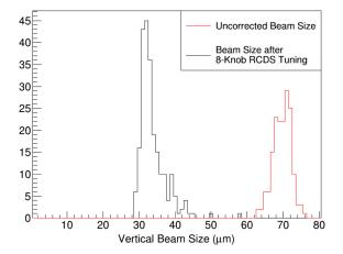
FIG. 5. Histogram of hundreds of experimental vertical beam size measurements both using the standard lattice for light-source operations with no additional tuning and after tuning with the RCDS algorithm using the best 8 eigenparameters. A clear improvement is observed. Note also the high-side tail of the low-beam-size distribution.
