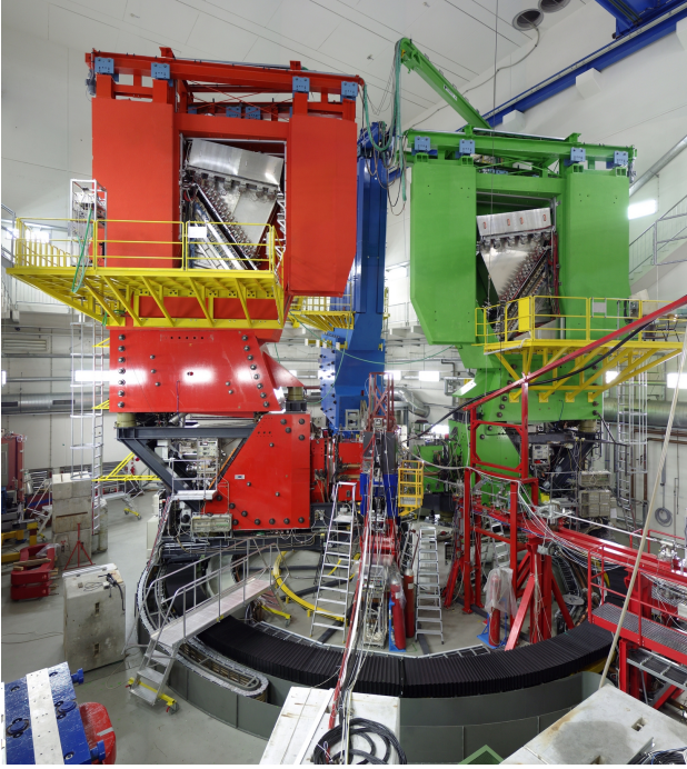
FIG. 12 (Color online) Top: the schematics of the three-spectrometer setup of the A1 experiment at Mainz, and a photo is shown at the bottom in which Spectrometer A, B and C are shown in red, blue and green respectively. The electron beam is from right to left (figure credit: Arnd P. Liesenfeld (top), and Markus Weis (bottom)).
