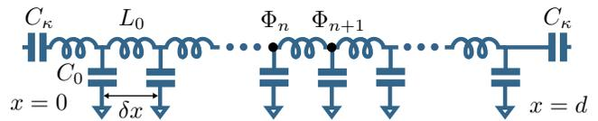
FIG. 3 Telegrapher model of an open-ended transmission line resonator of length  $d$ .  $L_0$  and  $C_0$  are, respectively, the inductance and capacitance associated to each node  $n$  of flux  $\Phi_n$ . The resonator is coupled to external transmission lines (not shown) at its input and output ports via the capacitors  $C_\kappa$ .
