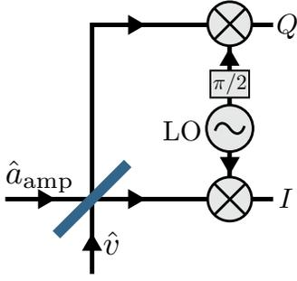
FIG. 16 Schematic representation of an IQ mixer. The RF signal  $\hat{a}_{\text{amp}}$  is split into two parts at a power divider, here illustrated as a beam splitter to account for added noise due to internal modes. Ideally, only vacuum noise  $\hat{v}$  is introduced at that stage. The two outputs are combined with a local oscillator (LO) at mixers. By phase shifting the LO by  $\pi/2$  in one of the two arms, it is possible to simultaneously measure the two quadratures of the field.
