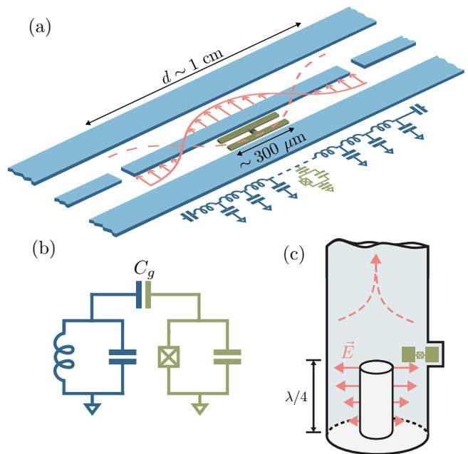
FIG. 7 Schematic representation of a transmon qubit (green) coupled to (a) a 1D transmission-line resonator, (b) a lumped-element LC circuit and (c) a 3D coaxial cavity. Panel (a) is adapted from Blais *et al.* (2004) and panel (c) from Reagor *et al.* (2016).
