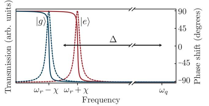
FIG. 19 Resonator transmission (dashed lines) and corresponding phase shifts (full lines) for the two qubit states (blue: ground; red: excited). When driving the resonator close to its pulled frequencies, the resonator response strongly depends on the state of the qubit. Adapted from (Blais *et al.*, 2007).
