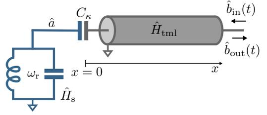
FIG. 11 LC circuit capacitively coupled to a semi-infinite transmission line used to model both damping and driving of the system. Here,  $\hat{b}_{\text{in}}(t)$  and  $\hat{b}_{\text{out}}(t)$  are the oscillators input and output fields, respectively.
