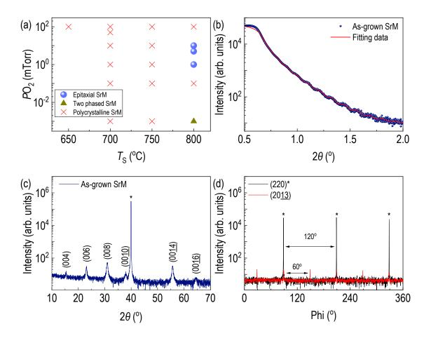
**Fig. 2.** (a) Growth phase diagram of  $SrFe_{12}O_{19}$  (SrM) epitaxial thin films on (111)  $SrTiO_3$ . Only filled blue circles are the condition for epitaxial thin films. (b) X-ray reflectivity and its fitting of epitaxial SrM thin film grown at the optimal growth condition. (c) X-ray diffraction of the epitaxial SrM thin film on (111)  $SrTiO_3$ . (d) Phi scans of (220)  $SrTiO_3$  and (2013) SrM epitaxial thin film.
