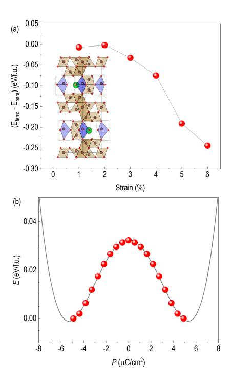
**Fig. 6.** (a) Energy difference between ferroelectric and paraelectric phase versus compressive strain. Inset shows atomic structure in stabilization of ferroelectric phase. (b) Energy versus polarization curve in stabilization of ferroelectric phase. Clear double well potential is built.
