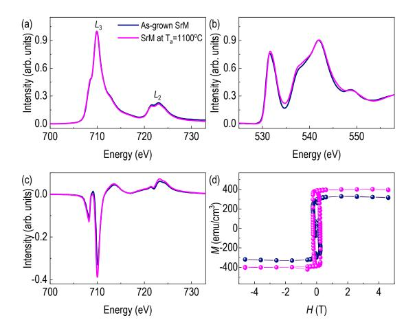
**Fig. 4.** X-ray absorption results are seen: (a) Fe *L*-edge spectra and (b) O *K*-edge spectra of asgrown and annealed SrM epitaxial thin films. (c) X-ray magnetic circular dichroism of as-grown and annealed SrM epitaxial thin films at 0.5 T and 300 K. (d) Magnetic hysteresis curves of asgrown and annealed SrM epitaxial thin films at room temperature, when the magnetic field is parallel to film surface normal.
