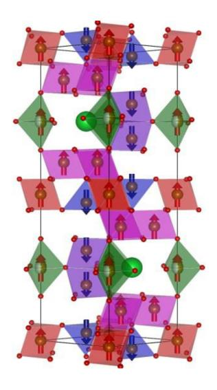
Fig. 1. Atomic structure of  $SrFe_{12}O_{19}$
