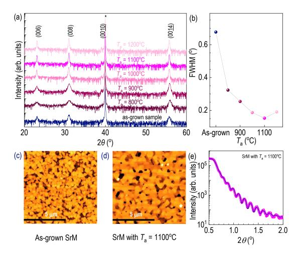
**Fig. 3.** (a) X-ray diffraction of epitaxial SrM thin films annealed at different temperatures in air. (b) Full width half maximum of rocking curves from  $00\underline{14}$  diffraction of SrM. Topographic images of (c) the as-grown SrM and (d) SrM annealed at  $1100^{\circ}$ C. (e) X-ray reflectivity and its fitting of SrM annealed at  $1100^{\circ}$ C.
