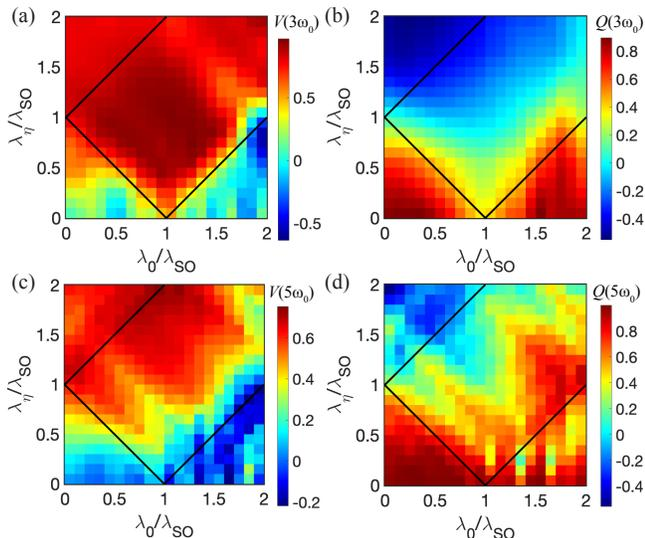
Figure 4. Topology fingerprints in the polarization state. Phase diagram of the Stokes parameters (a), (c)  $V$  for circular and (b), (d)  $Q$  for linear polarization for the 3rd (top) and 5th (bottom) harmonics.
