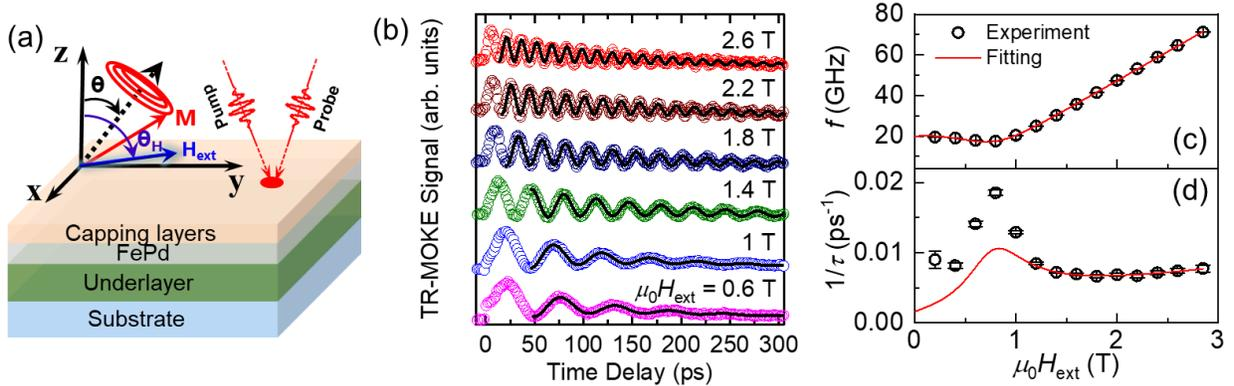
FIG. 2. (a) The schematics of sample stack and TR-MOKE measurement configurations ( $\theta_H \approx 80^\circ$ ). (b) TR-MOKE signals (symbols) measured on Cr/Pt/FePd(8) under varying  $H_{\text{ext}}$  at RT and their fitting curves (solid lines). (c) and (d) An example of fitting  $f$  vs.  $H_{\text{ext}}$  and  $1/\tau$  vs.  $H_{\text{ext}}$  to extract  $H_{k,\text{eff}}$  and  $\alpha$  from Cr/Pt/FePd(8). Circles and curves represent experimental data and modeling fitting, respectively.
