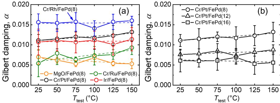
FIG. 4. Gilbert damping as a function of  $T_{\text{test}}$  for (a) 8-nm FePd samples and (b) Pt-seeded FePd samples. In (a) and (b), symbols represent experimental data and dashed lines are corresponding linear fittings that are used to calculate the change of  $\alpha$  (denoted as  $\Delta\alpha$ ) in Figure 5.
