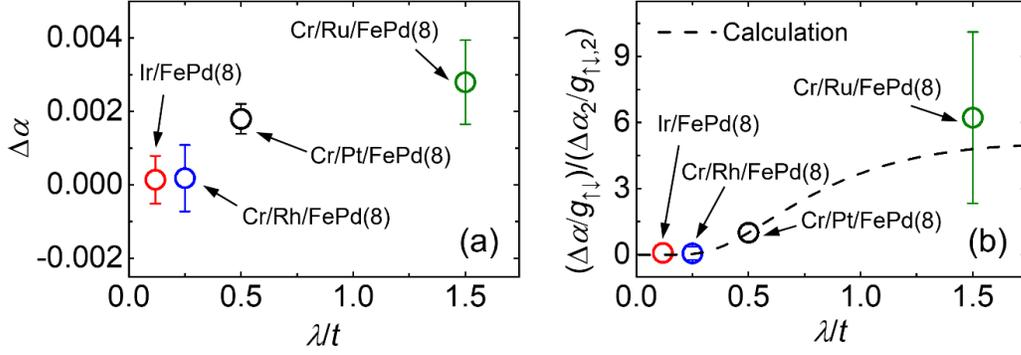
FIG. 5. (a) The change of  $\alpha$  vs. the spin-diffusion length  $\lambda$  normalized to the buffer-layer thickness  $t$  [ $\Delta\alpha = \alpha(150\text{ }^\circ\text{C}) - \alpha(25\text{ }^\circ\text{C})$ ]. (b) Comparison of the theoretically predicted (dashed line) and experimentally measured (symbols) trend for  $(\Delta\alpha/g_{\uparrow\downarrow})/(\Delta\alpha_2/g_{\uparrow\downarrow,2})$  vs.  $\lambda/t$ .
