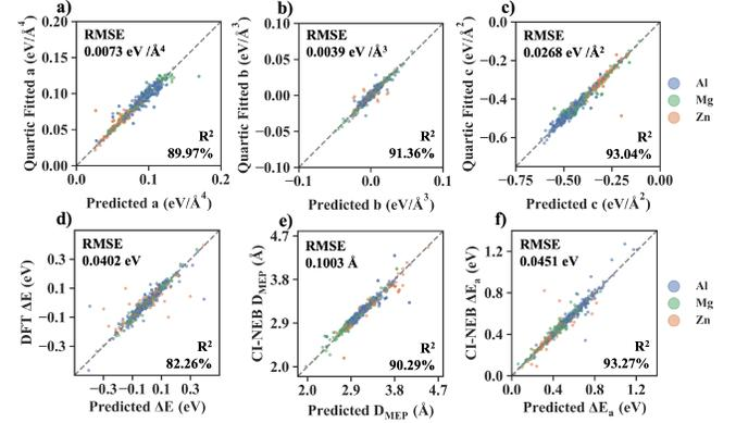
FIG. 8. Performances of surrogate models to predict vacancy migration energetics based on Eq. (5). (a)-(c): Comparisons between directly fitted results and predictions from our surrogate models for  $E_{\text{MEP}}(x)$  coefficients ( $a$ ,  $b$ , and  $c$  in Eq. (5)). (d)-(f): Comparisons between DFT+CI-NEB calculated results and predictions based on our surrogate-model-predicted  $E_{\text{MEP}}(x)$  for  $\Delta E$  (d),  $D_{\text{MEP}}$  (e), and  $\Delta E_a$  (f).
