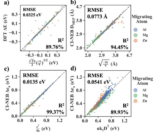
FIG. 6. Methods to estimate  $\Delta E$  (a),  $D_{\text{MEP}}$  (b), and  $\Delta e_a$  (c) of vacancy migration MEPs. (a)-(c) Comparisons between DFT+CI-NEB calculated  $\Delta E$  (a),  $D_{\text{MEP}}$  (b), and  $\Delta e_a$  (c) and those estimated based on Eq. (5) and Eq. (8). (d) Correlations between DFT+CI-NEB calculated  $\Delta e_a$  and  $k_f D^2$  to verify Eq. (9).
