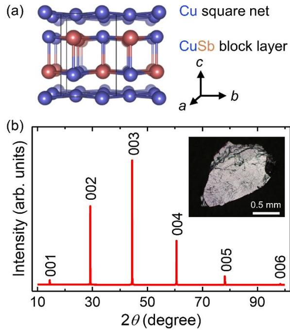
FIG. 1. (a) Crystal structure of  $\text{Cu}_2\text{Sb}$ . (b) XRD pattern of  $\text{Cu}_2\text{Sb}$  single crystal. Inset shows the photograph of  $\text{Cu}_2\text{Sb}$  single crystal cleaved along  $ab$ -plane.
