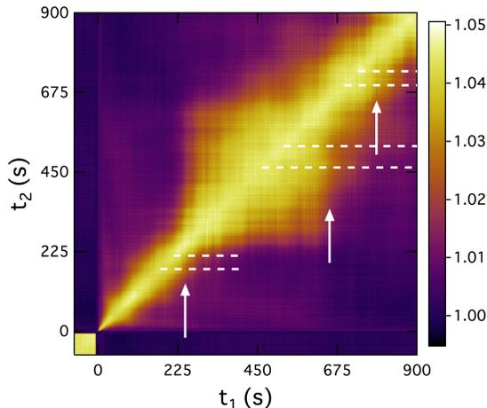
FIG. 7. Instantaneous correlation function  $C(q_\omega, t_1, t_2)$  during a stress relaxation measurement following a step to  $\gamma = 6\%$  at  $q_\omega = 0.26 \text{ nm}^{-1}$  along the vorticity direction. The arrows indicate waiting times at which intermittent events cause loss of correlation. The dashed lines show the boundaries of the regions over which averages were performed to obtain the correlation functions at fixed  $t_2$  shown in Fig. 10.
