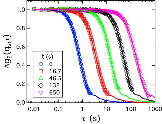
FIG. 12. Normalized autocorrelation functions at waiting times  $t = 6$  s (circles), 16.7 s (squares), 46.5 s (triangles), 132 s (diamonds), and 650 s (inverted triangles) after a step to 6% strain. The solid lines show results of fits based on convective dynamics modeled by the parabolic velocity profile given in Eq. (9).
