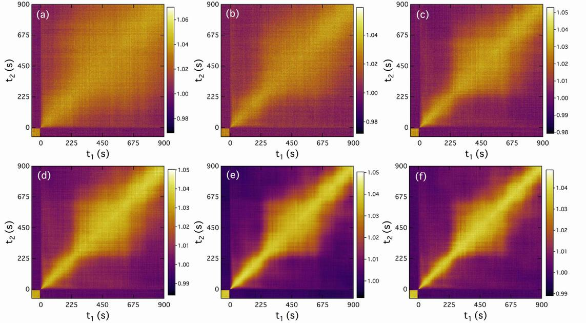
FIG. 9. Instantaneous correlation function  $C(q_\omega, t_1, t_2)$  during stress relaxation measurements following a step to strain of 6% measured along the vorticity direction at (a)  $q_\omega = 0.09$  nm $^{-1}$ , (b)  $q_\omega = 0.15$  nm $^{-1}$ , (c)  $q_\omega = 0.18$  nm $^{-1}$ , (d)  $q_\omega = 0.21$  nm $^{-1}$ , (e)  $q_\omega = 0.24$  nm $^{-1}$ , (f)  $q_\omega = 0.30$  nm $^{-1}$ .
