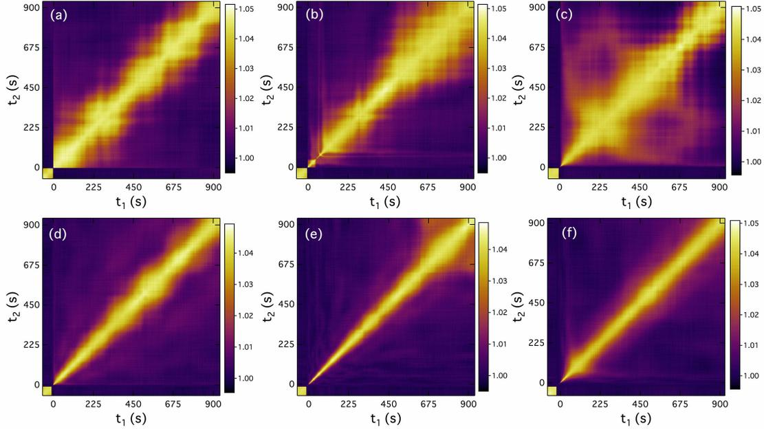
FIG. 8. Instantaneous correlation function  $C(q_\omega, t_1, t_2)$  during stress relaxation measurements following steps to strains of (a) 2%, (b) 4%, (c) 5%, (d) 8%, (e) 12%, and (f) 20% measured at  $q_\omega = 0.26 \text{ nm}^{-1}$  along the vorticity direction, perpendicular of the initial strain.
