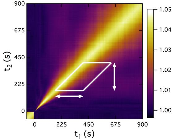
FIG. 3. Instantaneous correlation function  $C(q_v, t_1, t_2)$  during a stress relaxation measurement following a step to  $\gamma = 6\%$  measured at  $q_v = 0.26 \text{ nm}^{-1}$  along the direction of the initial strain. The white parallelogram indicates the region employed in calculating the autocorrelation function at  $t = 293 \text{ s}$ . The arrows, indicating the size of the region, span  $171 \text{ s} < t_{1,2} < 415 \text{ s}$ .
