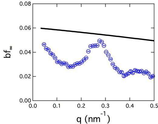
FIG. 4. The product  $bf_\infty$  (symbols) obtained from the amplitude of the XPCS correlation function,  $g_2(\mathbf{q}, \tau) - 1$ , at small  $\tau$  measured on the soft glass. The line shows the Sievert factor  $b$  obtained from a separate XPCS measurement on a thin aerogel sample<sup>32</sup>. The wave-vector-dependent non-ergodicity parameter  $f_\infty$  is a measure of the fourier components of the arrested concentration fluctuations in the glass<sup>33</sup>
