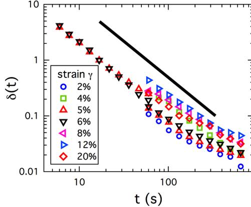
FIG. 11. Factors used to scale  $\tau$  in order to collapse  $\Delta g_2(q_v, \tau; t)$  at different waiting times like in Fig. 5(b). The correlation functions at all waiting times and all strains, as indicated in the legend, were scaled with respect to that for 6% strain at  $t = 15$  s. Each value of  $\delta$  is an average of the factors over wave vectors  $0.024 \text{ nm}^{-1} < q < 0.030 \text{ nm}^{-1}$ . The solid line depicts the power-law relation  $\delta \sim t^{-1.2}$ .
