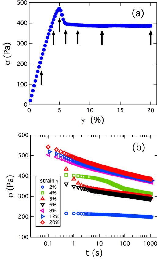
FIG. 1. (a) Stress as a function of strain during start-up shear at  $\dot{\gamma} = 0.01 \text{ s}^{-1}$ . The arrows indicate the strain values at which shear was stopped and strain held fixed in the stress relaxation measurements. (b) Stress as a function of waiting time with strain held at these various values following a step from zero strain at strain rate  $\dot{\gamma} = 0.01 \text{ s}^{-1}$ .
