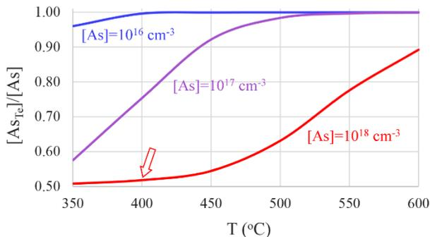
Figure 8. Fraction of  $As_{Te}$  defects formed at Stage 2 as a function of annealing temperature and total As concentration. Red arrow shows the conditions used in simulation on Figure 6.
