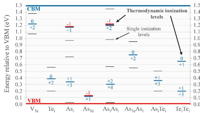
Figure 2. Ionization levels of defect and complexes. Thick lines with numbers show thermodynamic ionization levels and corresponding charge states, thin lines show single ionization levels for secondary charge states.
