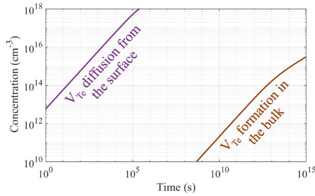
Figure 4. Kinetics of  $V_{Te}$  accumulation at 450°C by Frenkel pair formation and due to diffusion from the surface. Diffused concentrations shown at  $1\mu m$  from the surface.
