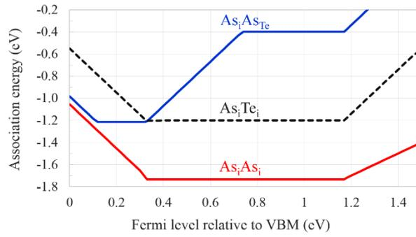
Figure 3. Association energies of the most important As-related complexes calculated taking into account the most stable states of complexes and separate point defects at a given Fermi level (see Eq.8 in our previous work [29]). The horizontal lines indicate defect association without the change of charge state; the inclined lines indicate association with the change of charge state.
