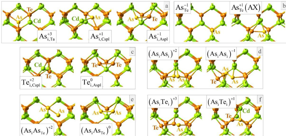
Figure 1. Atomic structure of the most stable configuration of defects and complexes in different charge states: (a)  $As_i$  defect, (b)  $As_{Te}$  defect, (c)  $Te_i$  defect, (d)  $(As_i As_i)$  complex, (e)  $(As_i As_{Te})$  complex, (f)  $(As_i Te_i)$  complex.
