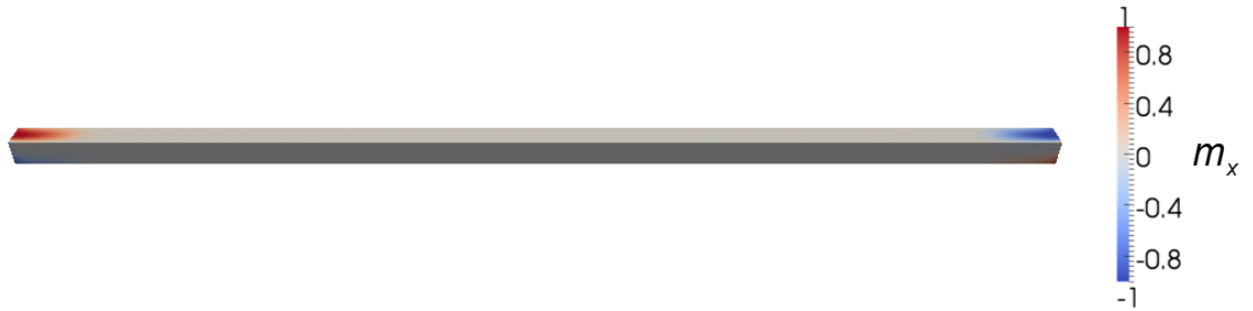
Figure 10: Remanent largely uniform longitudinally magnetized domain state obtained at T = 273 K with bulk magnetic properties.
