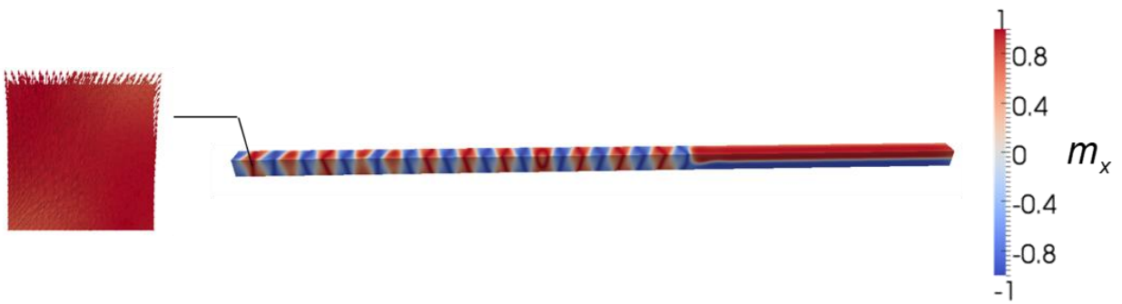
Figure 13. Periodic array of domains obtained in the presence of negative uniaxial anisotropy ( K_u = -1.0 \text{ Merg/cm}^3 ) at reduced saturation magnetization of M_s = 250 \text{ emu/cm}^3 .
