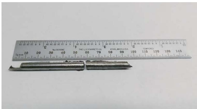
FIG. 1. A typical 15-g, ~5-mm in diameter ingot of  $\text{Al}_x\text{Fe}_2\text{B}_2$  alloys synthesized by arc-melting followed by suction casting.
