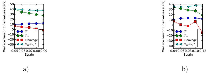
FIG. 5. The elastic stability criteria plotted as a function of strain for the D0<sub>3</sub> and L6<sub>0</sub> structures at a composition of 75 at. % Mg (FIGs. 5a and 5b respectively). The plot shows that a failure via cleavage occurs at a strain of approximately 9% for the D0<sub>3</sub> structure and a strain of 8% for L6<sub>0</sub>.
