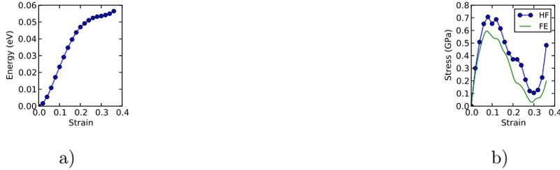
FIG. 6. The stress-strain and energy-strain relation for the  $D0_3$  structure under a  $\langle 100 \rangle$  type tensile load. Only the tetragonal path is explored in this simulation. In FIG. 6b “Hellmann-Feynman” refers to the stresses obtained directly from VASP using the Hellman-Feynman theorem and “Fitted from Energy” refers to the stresses obtained by taking the derivative of energy per unit volume with respect to strain.
