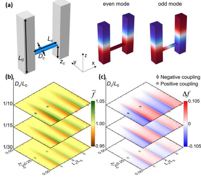
FIG. 2. (a) The eigenmodes of the two acoustic cavities coupled with an air channel. The normalized eigenvalue mean  $\bar{f}$  (b) and eigenvalue splitting  $\Delta f$  (c) as functions of  $L_c$  and  $z_c$ , and for different  $D_c$ . The diamonds and stars mark the geometric values chosen for our acoustic HOTP design.
