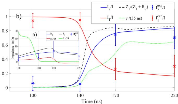
FIG. 5. Simulation of the lumped-circuit equation (LCE) a) the abrupt decrease of the LDP resistance  $R_2$  (green) enables the current transfer, b) the evolution of the current partition  $I_2/I$  (blue) follows the impedance ratio (dashed black) with a delay of the current transfer time (dotted green).
