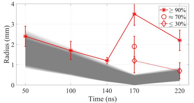
FIG. 3. Gray: location of the plasma with  $n_e > 0.1 n_{e,max}$  (from continuum radiation intensity) with uncertainty in light gray. Red: locations at which a certain percentage of the discharge current was measured. At  $t \geq 170$  ns the measurements were obtained in an LDP with a density lower than 10% of  $n_{e,max}$ . Initially, the current implodes together with the main plasma, while at stagnation (140 ns to 170 ns), a sudden current redistribution to much larger radii takes place.
