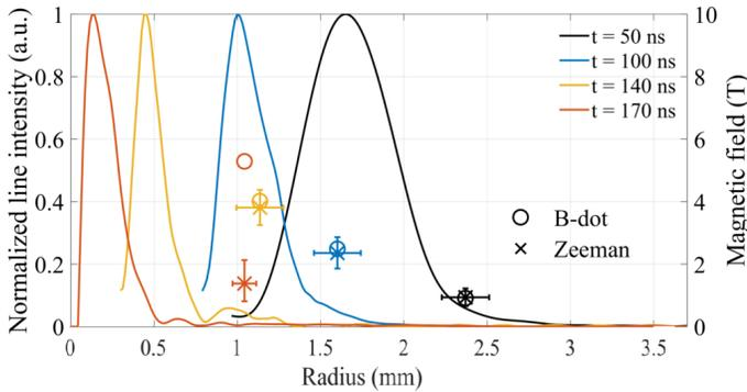
FIG. 2. Evolution of the O IV ( $t = 50$  ns) and O VI ( $t \geq 100$  ns) emission intensity radial distribution along with the magnetic field measured at the outer chord: at  $t = 50$  ns to 140 ns, the agreement between expected (B-dot) and measured magnetic field (Zeeman) indicates the confinement of the entire discharge current in the imploding plasma. At  $t = 170$  ns the fraction of the current that can be located in the stagnating plasma is  $\lesssim 30\%$ .
