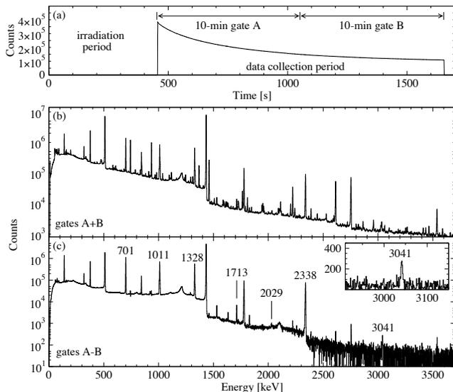
FIG. 2. (a) Time spectrum from the ADC clock recorded with each  $\gamma$ -ray event illustrating the irradiation and out-of-beam collection period split into two parts, gates A and B. Lower panels show (b) the total  $\gamma$ -ray spectrum recorded (gate A plus gate B) and (c) the subtracted spectrum (gate A minus gate B) described in the text. The inset spectrum is on a linear scale and expands the region near the 3041-keV,  $E6$  transition.
