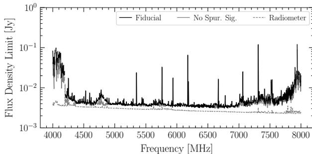
Figure 3. A comparison of the derived flux density sensitivities (with and without the inclusion of the spurious signal nuisance parameter correction) compared with the radiometer equation expected sensitivity. For presentation, the limits have been smoothed with a median filter.
