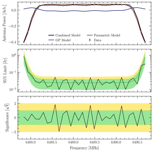
Figure 2. (*Top*) An illustration of the data and the fitted components of our model for a single coarse channel. (*Middle*) The 95% CL upper limits on a flux density excess with bandwidth  $\delta f = 91.6$  kHz. (*Bottom*) The corresponding significances of the flux density excesses and deficits.
