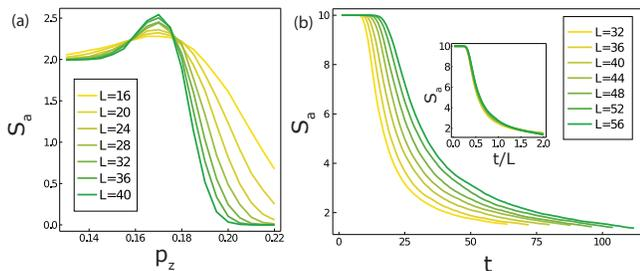
FIG. 3. (a) The ancilla EE  $S_a$  measured at  $t = L$  as a function of  $p_z$  for fixed  $p_u = 0.01$  in the hybrid random circuit. (b)  $S_a$  as a function of time at  $(p_z, p_u) = (0.17, 0.01)$  in the hybrid random circuit. The inset is the same, plotted as a function of  $t/L$ .
