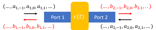
FIG. 1. Dynamically-modulated two-port system. The fields at each port consist of multiple frequency sidebands.
