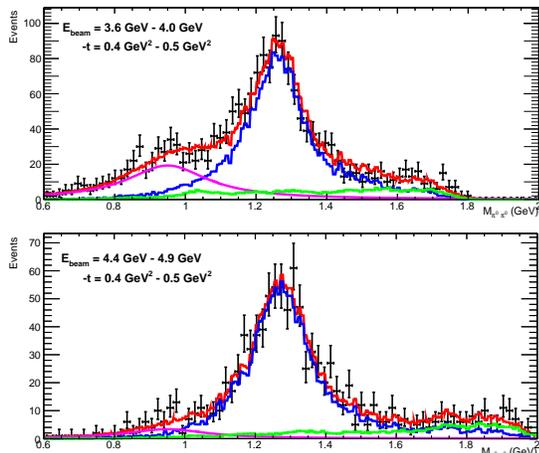
FIG. 2. Result of the maximum likelihood binned fit to the  $\pi^0\pi^0$  invariant mass distribution for two representative bins, as reported in the panels. The red curve is the full fit PDF, while the blue, green, and violet curves represent, respectively, the  $f_2$  signal PDF, the phase-space background PDF, and the low-mass background PDF including the region of the  $f_0(980)$  meson.
