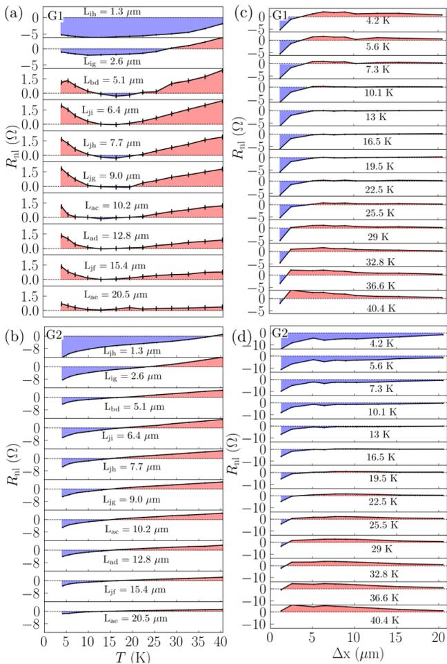
FIG. 2. (a,b) Experimental nonlocal resistance  $R_{nl}$  vs  $T$  for each  $L_{\alpha\beta}$  for (a) G1 and (b) G2. (c,d)  $R_{nl}$  vs  $\Delta x$  for each  $T$  for (c) G1 and (d) G2. The dotted lines indicate  $R_{nl} = 0$ , with negative (positive) regions of  $R_{nl}$  shaded in blue (red).
