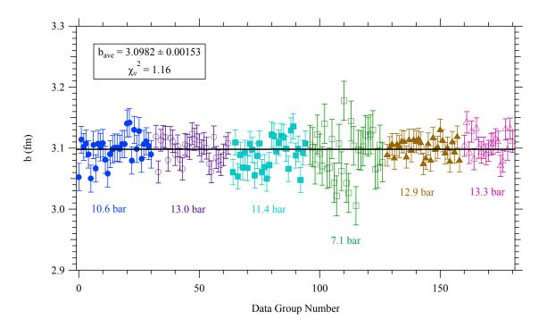
FIG. 4. Bound neutron scattering length for the six data sets after all corrections, fit to a constant. Error bars are due to Poisson counting statistics from the  $\Phi_D$  data only.
