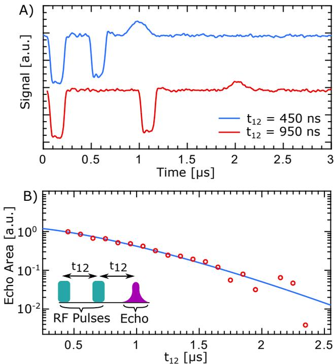
FIG. 2. A) Optically detected electron spin echoes in the  ${}^4I_{13/2}$  excited state for different pulse delays with  $T = 1.9$  K and  $B = 8.7$  mT. B) Measurement (circles) and fit (line) of echo decay at 1.9 K, giving  $T_2 = 1.6 \pm 0.2 \mu\text{s}$  and  $x = 1.4 \pm 0.2$ . Inset: RF pulse sequence.
