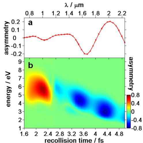
Figure 4: (color online) (a) Calculated energy integrated asymmetry amplitude in the BS channel for various laser wavelength assuming a 3.5-cycle pulse. (b) Calculated asymmetry map for the RCE channel as a function of kinetic energy and recollision time (corresponding to the wavelength given on the top axis).
