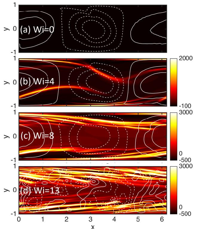
FIG. 20. Snapshots of the finite amplitude Tollmien-Schlichting wave solution at  $Re = 10000$  and (a)  $Wi = 0$ , (b)  $Wi = 4$ , (c)  $Wi = 8$ , (d)  $Wi = 13$  [307]. White contours are wall-normal velocity and colors are deviations of  $xx$  polymer stretch from laminar values.
