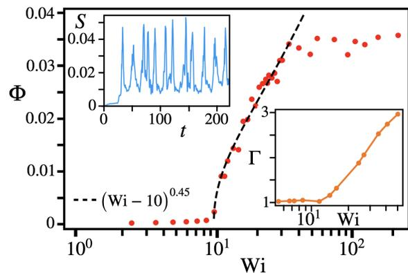
FIG. 6. Order parameter  $\Phi = \overline{S(t)}$  versus Weissenberg number  $Wi$ . The dashed line indicates the fitted scaling law beyond the elastic instability. Upper inset: Secondary flow strength  $S(t)$  plotted versus  $t$  for  $Wi = 16.3$ . Lower inset: Flow resistance quantified by the azimuthal stress on the outer cylinder plotted versus  $Wi$ . Adapted from Ref. [154] with permission from *EPL*; copyright (2018).
