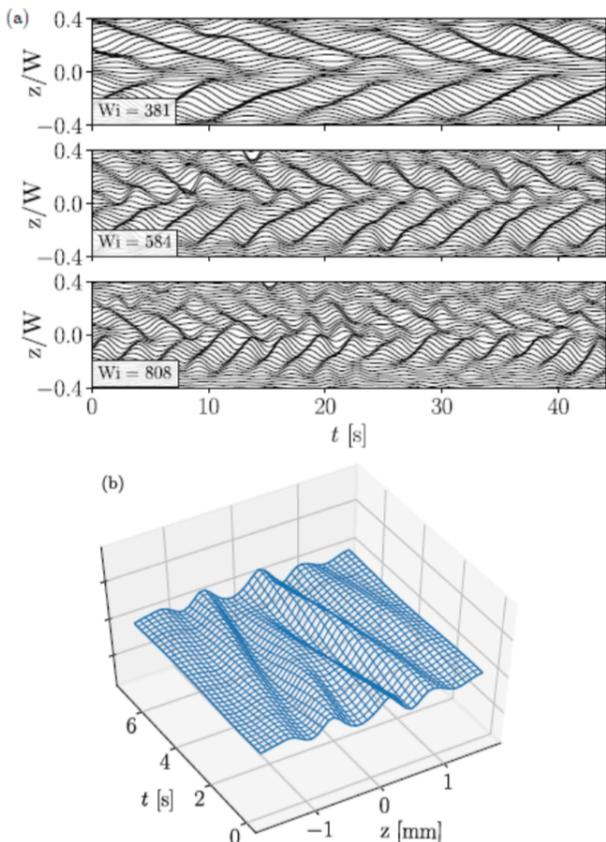
FIG. 11. (a) Space-time plots at  $-0.4 < z/W < 0.4$  of the stream-wise velocity fluctuations,  $u'(z, t)$  exhibiting elastic wave structures for three values of  $Wi$ . The time series are filtered via a band-pass Butterworth filter centered on the spectral peaks to remove background noise. (b) Stream-wise velocity, phase averaged at the elastic wave frequency for  $Wi = 407$  [200].
