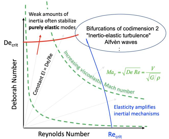
FIG. 4. Sketch of a canonical stability diagram for representing the onset of viscoelastic flow instabilities in a complex fluid.
