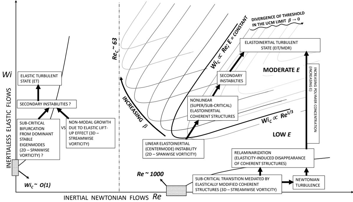
FIG. 21. Schematic representation of various transition scenarios for viscoelastic pipe flow in the  $Re$ - $Wi$  plane. The laminar flow is characterized by the Poiseuille velocity profile with rectilinear streamlines. The linearly unstable regions in the interior of the  $Wi$ - $Re$  plane, corresponding to the center-mode instability, are marked by a thick black line (solid) for one specific values of  $\beta$ , while those for other values of  $\beta$  are depicted by light gray lines.
