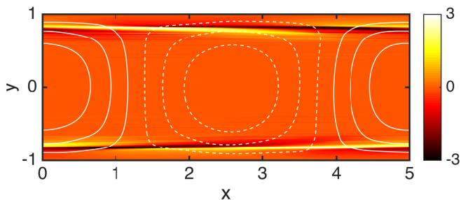
FIG. 19. Snapshot of the finite amplitude Tollmien-Schlichting wave solution at  $Re = 3000$ ,  $Wi = 10$  [306]. White contours are wall-normal velocity, colors are deviations of  $xx$  polymer stretch from laminar values. Reproduced with permission from [306].
