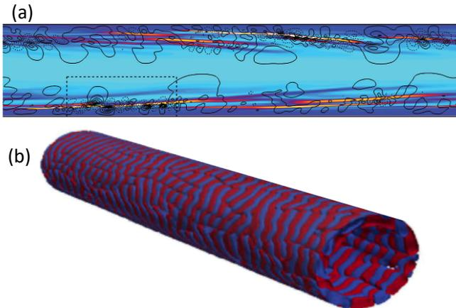
FIG. 18. Snapshots of simulations of EIT in (a) channel flow [300] and (b) pipe flow [299]. In (a) color contours indicate polymer stretching and lines indicate the magnitude  $Q$  of the second invariant of the velocity gradient tensor; reproduced with permission from [300]. In (b) isosurfaces indicate  $Q$ ; ; licensed under a Creative Commons Attribution (CC BY) license.
