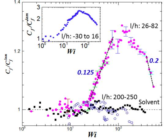
FIG. 10. Dependence of the normalized friction factor  $C_f/C_f^{lam}$  on  $Wi$  for three values of non-dimensional distance from the third layer of cylinders (at  $l/h = 0$ )  $l/h$ : (i) -30 to 16 (inset), (ii) 26 to 82 (filled circle), (iii) 200 to 250 (open circle), and (iv) Newtonian solvent 26 to 82 (filled black square). Inset shows  $C_f/C_f^{lam}$  versus  $Wi$  across three rows of cylinders [198].
