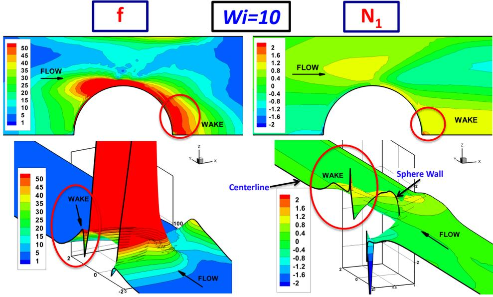
FIG. 26. Dimensionless fluidity and first normal-stress difference  $N_1$  in flow past a sphere (sphere-to-tube aspect ratio 1:2) of a WLM solution; solvent-fraction  $\beta = 5 \times 10^{-3}$  and moderate hardening features,  $Wi=10$ ; see López-Aguilar et al. [447] for further details of the rheology used.
