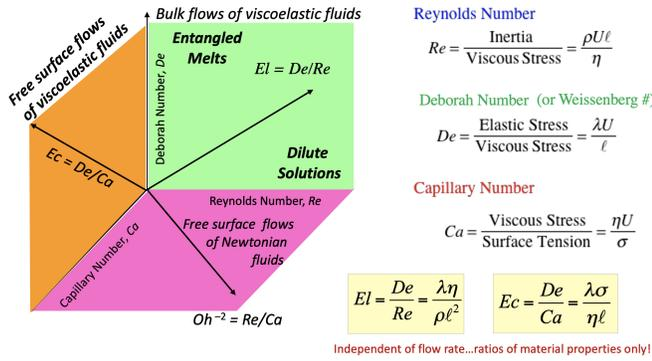
FIG. 3. A three-dimensional representation of the parameter space accessed in processing flows of complex fluids. Taking ratios of each pair of axes results in new dimensionless material parameters that are independent of the kinematics of the flow [75]. Note that here we have defined  $De$  as a ratio of stresses instead of the ratio of time scales presented in the text.
