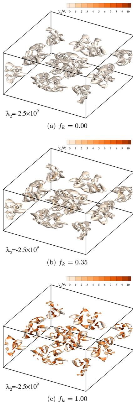
FIG. 17: Temporal evolution of the coherent and turbulent structures of the TGV at  $t = 6.5$  predicted with different  $f_k$  [40]. Vortical structures identified with the  $\lambda_2$  criterion [122].
