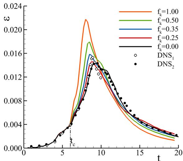
FIG. 15: Temporal evolution of the total kinetic energy dissipation,  $\varepsilon$  ( $\text{s}^{-1}$ ), for predictions at different  $f_k$ .
