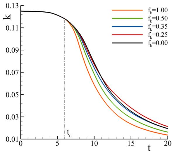
FIG. 14: Temporal evolution of the total kinetic energy,  $k$ , for predictions at different  $f_k$ .
