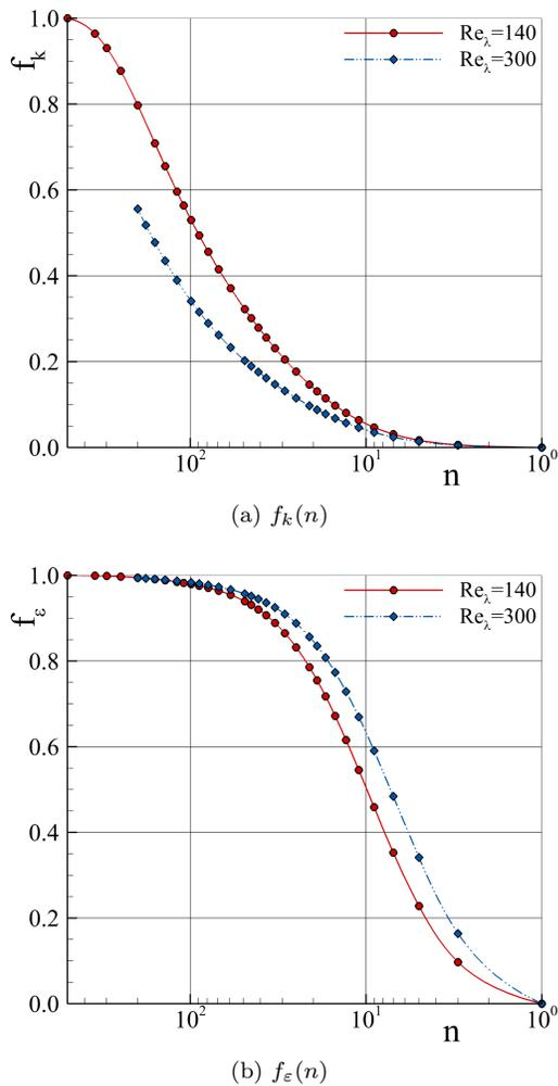
FIG. 4: Variation of  $f_k$  and  $f_\varepsilon$  with the relative filter size,  $n$ , at  $\text{Re}_\lambda = 140$  and  $300$ .
