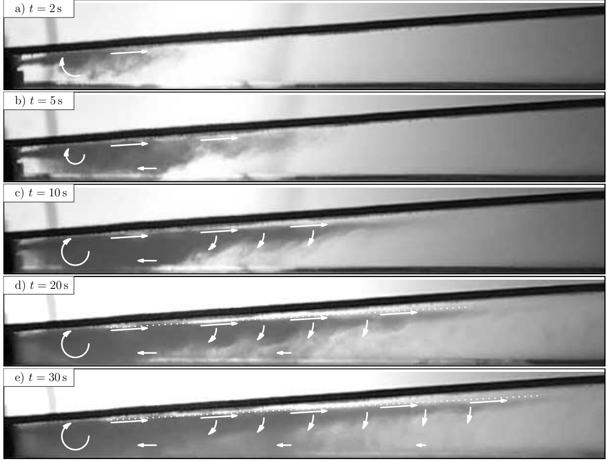
FIG. 3. [Multimedia online] Snapshots from Experiment 6 (with \theta = 4^\circ , d_p = 45 \mu\text{m} and \phi_0 = 0.01 ) showing the region extending 65 cm to the right of the source at 5 indicated times after the valve was opened. Superimposed white arrows qualitatively indicate the direction and speed of the flows. The dotted lines in d) and e) indicate the location of the settling front.
