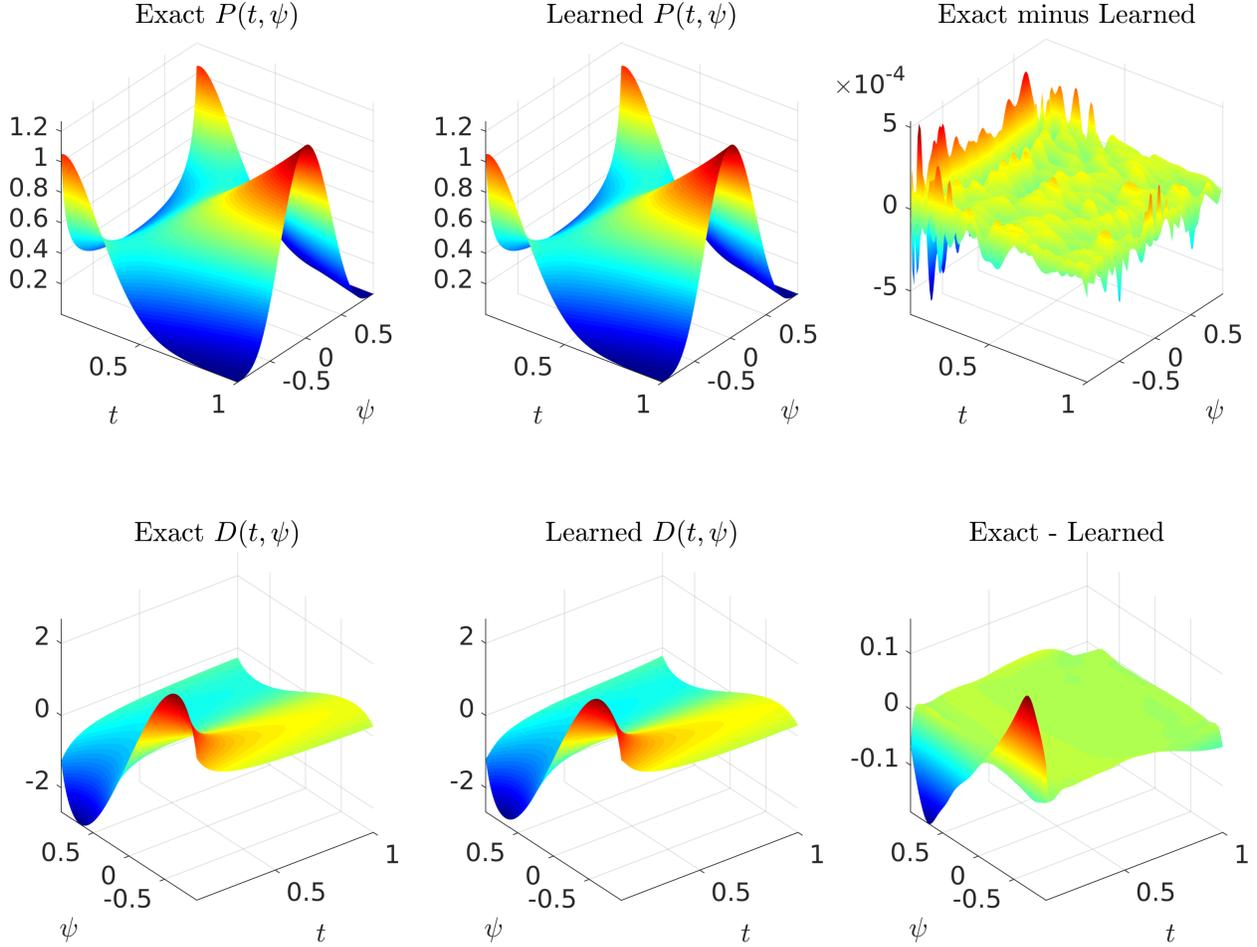
FIG. 3. *Conditional Expected Diffusion*: The exact probability density function  $P(t, \psi)$  alongside the learned one is depicted in the top panels, while the exact and learned conditional expected diffusion  $D(t, \psi)$  are plotted in the bottom panels. It is worth highlighting that the algorithm has seen no data whatsoever on the diffusion coefficient.
