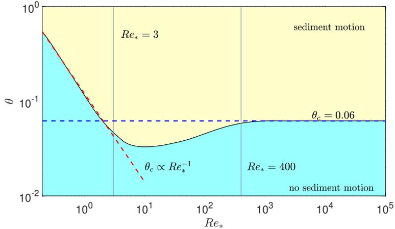
FIG. 2. Modified *Shields Diagram* fitted to the original data of Shields [9], where  $\theta_c \approx 0.06$  is independent of  $Re_*$  when  $Re_* > 400$  and  $\theta_c \propto Re_*^{-1}$  for  $Re_* < 3$ . An intermediate region defined by  $Re_* \in [3, 400]$  exists where  $\theta_c \in [0.02, 0.06]$  varies weakly and non-monotonically with  $Re_*$ .
