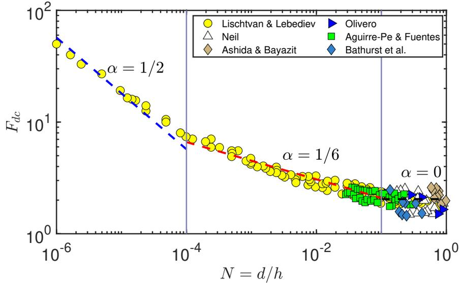
FIG. 3. The  $F_{dc} - N$  diagram with data reported by Ali and Dey [3, 26] along with the three scaling laws expressed as  $F_{dc} \sim N^{-\alpha}$  with  $\alpha = 1/2$ ,  $1/6$ , and  $0$  (in dashed lines). The original data sources are described in a number of studies that include Lischtvan and Lebediev [27], Neill [28], Ashida and Bayazit [29], Olivero [30], Aguirre-Pe and Fuentes [31], Bathurst *et al.* [32, 33].
