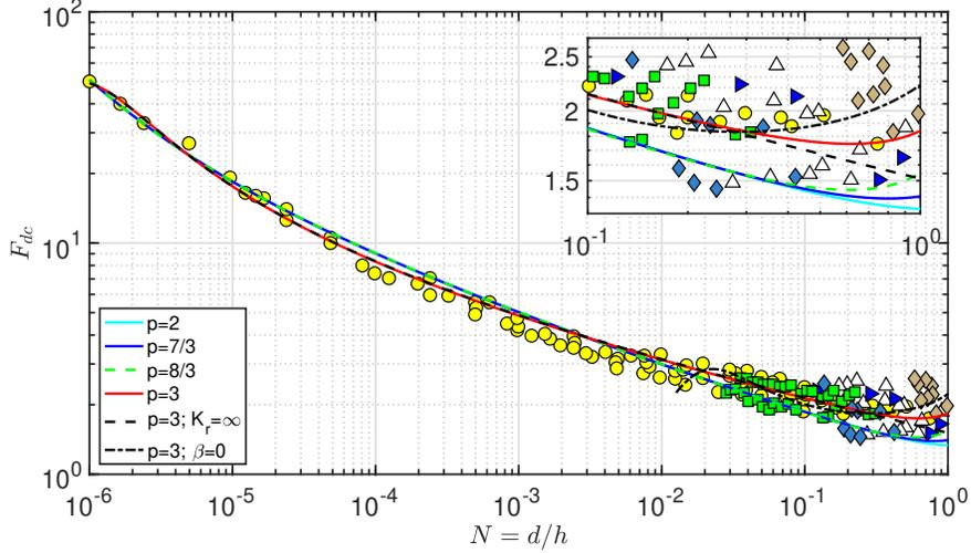
FIG. 5. Fitting the  $F_{dc} - N$  derived from the CSB model to the data in Figure 3. The inset is an enlarged frame associated with the large-roughness regime ( $N > 0.1$ ).
