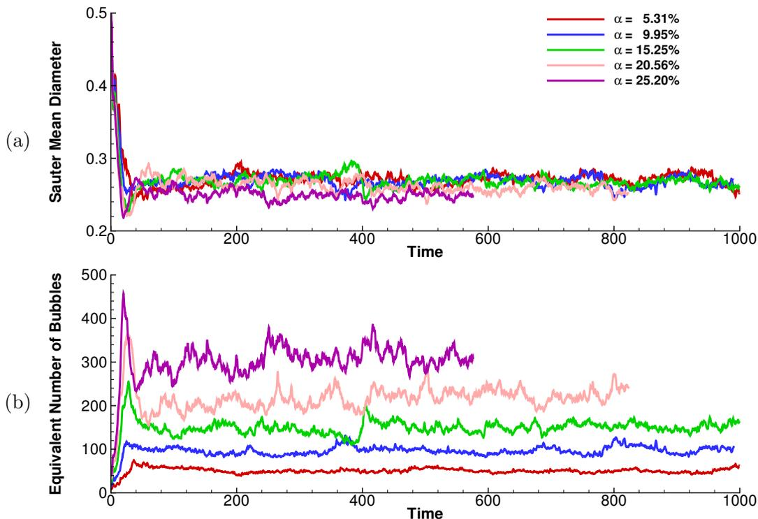
FIG. 3: (a) The Sauter Mean Diameter; (b) The equivalent number of bubbles, versus time for all five cases.
