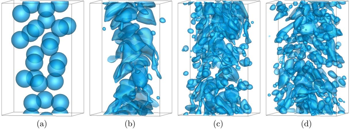
FIG. 1: Four frames showing the fluid interface for early times, 0.0(a), 10.0(b), 20.0(c) and 30.0(d), for void fraction equal to 15.25% (Case 3).
