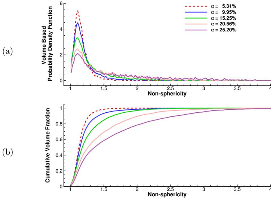
FIG. 11: The probability distribution of the light fluid blobs' non-sphericity for all cases. (a) The volume based probability density function, and (b) the cumulative volume fraction, at nearly steady state.
