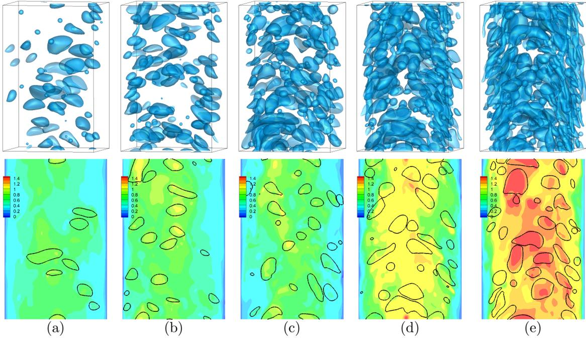
FIG. 5: The fluid interface at late times for all five cases in the top row and contours of the streamwise velocity in a plane through the middle of the channel in the bottom row.
