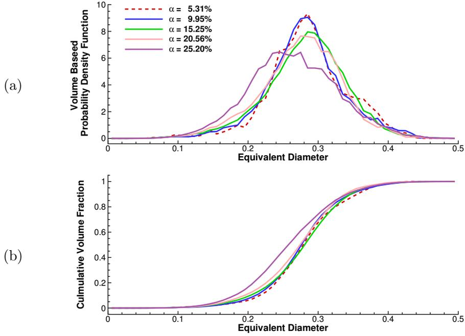
FIG. 10: The probability distribution of blob sizes of the light fluid for all cases. (a) The volume based probability density function, and (b) the cumulative volume fraction, at nearly steady state.
