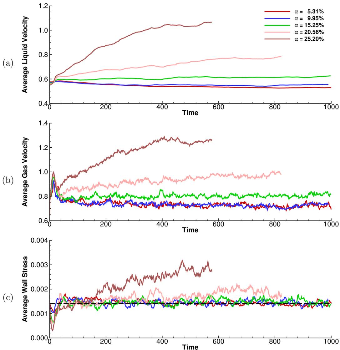
FIG. 2: (a) The liquid velocity; (b) The gas velocity; (c) The wall shear stress, versus time for all five cases. The dashed line in (c) is the equivalent wall shear stress balanced by  $\beta$ .
