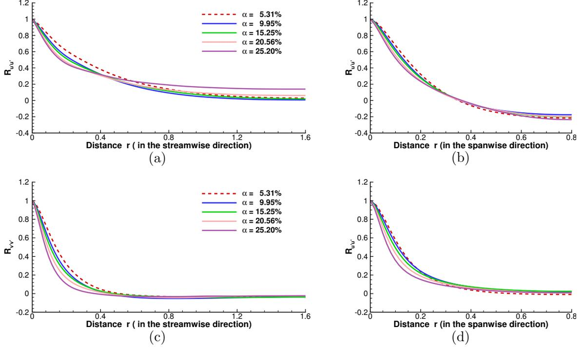
FIG. 14: The velocity conditional correlation functions. (a)  $R_{u'u'}$  in the streamwise direction; (b)  $R_{u'u'}$  in the wall-normal direction; (c)  $R_{v'v'}$  in the streamwise direction; (d)  $R_{v'v'}$  in the wall-normal direction.
