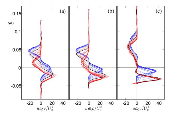
**Figure 9.** Time-averaged cross-stream distributions of vorticity flux in the wake (x/c = 1.05) for  $1 < u_f < 1$  for static model at  $\alpha = -5^\circ$  (a),  $3^\circ$  (b), and  $15^\circ$  (c). The traces are colored such black corresponds to the unactuated flow and increasing levels of red (blue) correspond to increasing levels of SS (PS) actuation.
