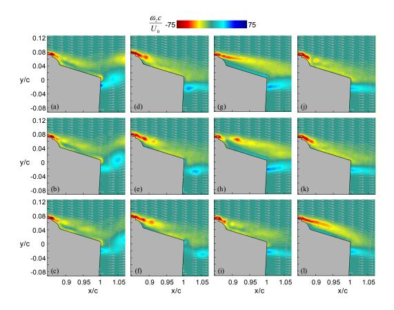
**Figure 13.** Raster plots of phase-averaged spanwise vorticity following actuation transitions at  $t/T_{\rm conv} = 0.3$ , 0.33, and 0.36: *PS-SS* (a – c), and *SS-PS* (d – f), and at  $t/T_{\rm conv} = 0$ , 0.07, and 0.46: 0-SS (g – i), and SS-0 (j – l).
