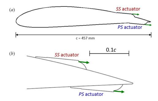
**Figure 2.** NACA4415 airfoil with modified profile geometry near the trailing edge (a), and a close-up of the trailing edge region (b).
