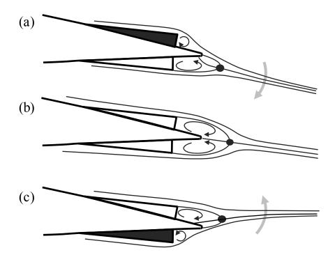
**Figure 1.** Conceptual bi-directional control of a pitching moment by hybrid formation and control of trapped vorticity at suction (a) and pressure (c) side of an airfoil tail. Passive formation of trapped vorticity is shown in (b).bvg
