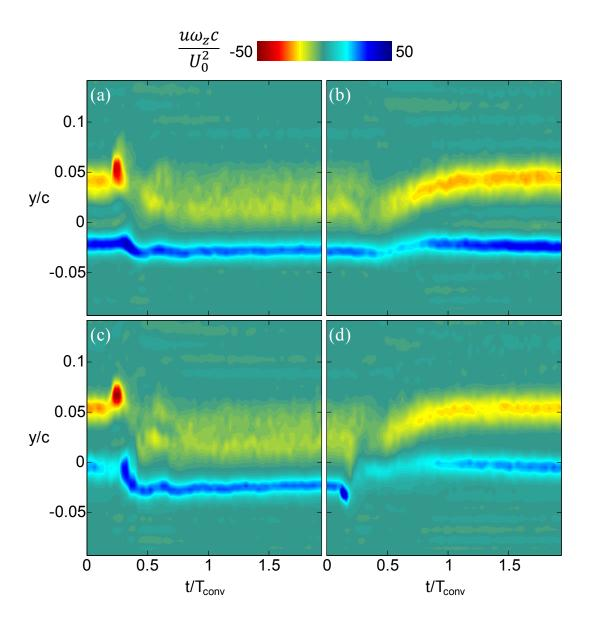
**Figure 14.** Color raster plots of time variation of the cross stream vorticity flux at x/c = 1.04 following transitions 0-SS (a), SS-0 (b), PS-SS (c), and SS -PS (d).
