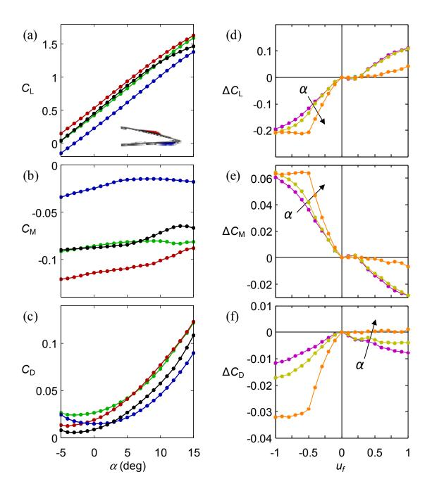
**Figure 5.** Variation of  $C_{\rm L}(a)$ ,  $C_{\rm M}(b)$ , and  $C_{\rm D}(c)$  with  $\alpha$  for the smooth airfoil ( $\bullet$ ) and modified  $[x_{\rm SS}=0.86{\rm c},x_{\rm PS}=0.95{\rm c}]$  airfoil with  $u_{\rm f}=0$  ( $\bullet$ ), 1 ( $\bullet$ ), and -1 ( $\bullet$ ). Variation of  $\Delta C_{\rm L}(d)$ ,  $\Delta {\rm CM}(e)$ , and  $\Delta C_{\rm D}(f)$  with  $u_{\rm f}$  for  $\alpha=0^{\circ}$  ( $\bullet$ ), 3° ( $\bullet$ ), and 15° ( $\bullet$ ).
