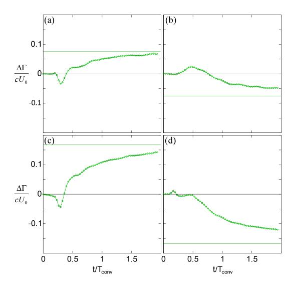
**Figure 16.** Time histories of the changes in circulation about the airfoil corresponding to the four actuation transition in Figure 14.
