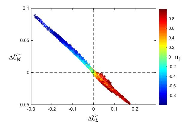
**Figure 7.** Variation of  $\Delta \widehat{C_M}$  with  $\Delta \widehat{C_L}$  for all the test cases:  $0.83 < x_{SS} < 1$ ,  $0.96 < x_{PS} < 1$ ,  $-5^\circ < \alpha < 15^\circ$ , and  $-1 < u_{\rm f} < 1$ .
