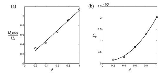
**Figure 3.** Synthetic jet calibration: variation of RMS jet velocity (a) and momentum coefficient (b) at the center of the jet orifice with the jet power fraction  $\mathcal{E}$ .
