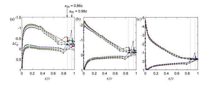
**Figure 4.** Distributions of static pressure Cp when the actuators are mounted at  $[x_{SS} = 0.86c, x_{PS} = 0.95c]$  for  $\alpha = 3 \circ (a)$ ,  $9 \circ (b)$ , and  $15 \circ (c)$ , and actuation level  $u_f = 0$  ( $\triangle$ ), 1 ( $\triangle$ ), and -1 ( $\triangle$ ). Corresponding  $C_p$  for the smooth airfoil (-).
