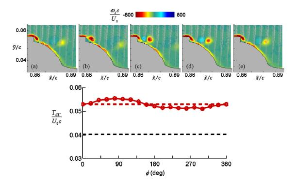
**Figure 10.** Raster plots of phase-averaged spanwise vorticity during the cycle of the synthetic jet at  $\phi = 0^{\circ}$  (a),  $80^{\circ}$  (b),  $160^{\circ}$  (c),  $240^{\circ}$  (d), and  $320^{\circ}$  (e), and the corresponding time history of circulation within the domain. Dashed lines indicate time-averaged circulation when  $u_{\rm f} = 0$  (black) and  $u_{\rm f} = 1$  (red).
