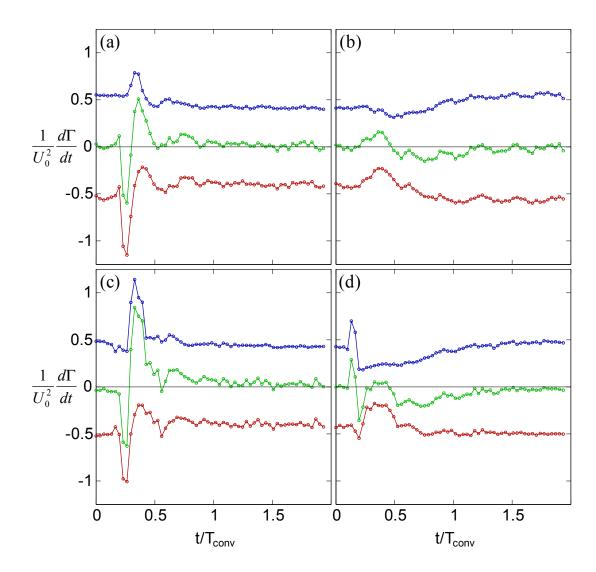
**Figure 15.** Respective time histories of vorticity flux of the four actuation transitions in Figure 14. Vorticity flux from suction and pressure sides of the airfoil is computed separately (red and blue traces, respectively). The total flux is shown in green.
