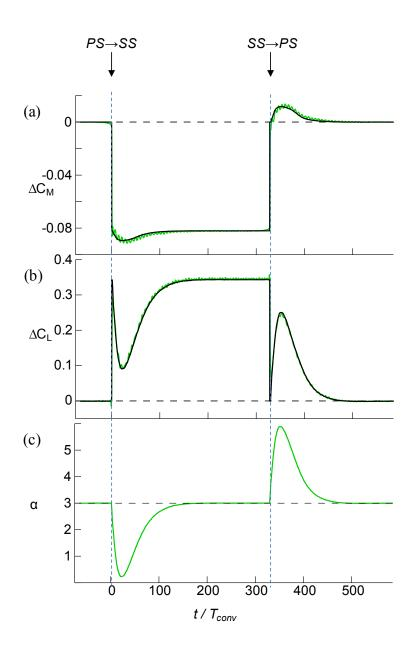
**Figure 11.** Time histories of  $\alpha$  (a),  $\Delta C_{\rm L}$  (b), and  $\Delta C_{\rm M}$  (c) during step changes in actuation between SS and PS actuators. Black traces indicate corresponding steady-state values based on a look up table using  $\alpha$  and  $u_{\rm f}$ .
