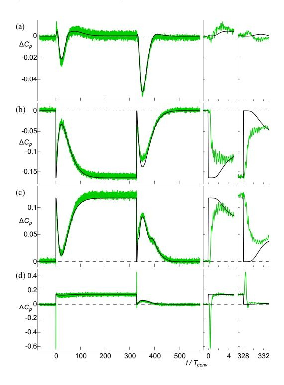
**Figure 12.** Time histories of  $\Delta C_p$  at the leading edge (a), on the suction surface at x/c = 0.39 (b), on the pressure surface at x/c = 0.4c (c), and at the trailing edge (d), with corresponding static values.
