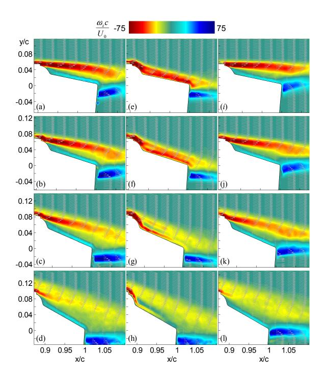
**Figure 8.** Raster plots of the time-averaged spanwise vorticity  $\omega_z c/U_o$  at  $\alpha = -3^\circ$  (a,e,i),  $3^\circ$  (b,f,j),  $9^\circ$  (c,g,k), and  $15^\circ$  (d,h,l) with  $u_f = 0$  (a-d), 1(e-h), and -1 (i-l).
