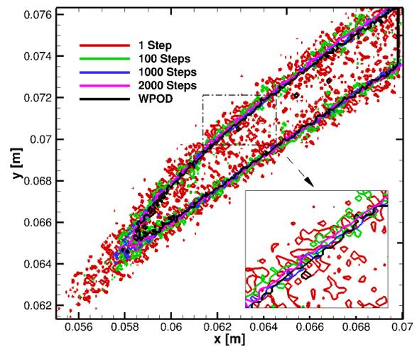
(d)Line comparison of the vibrational temperatures along the 3400 K constant line
