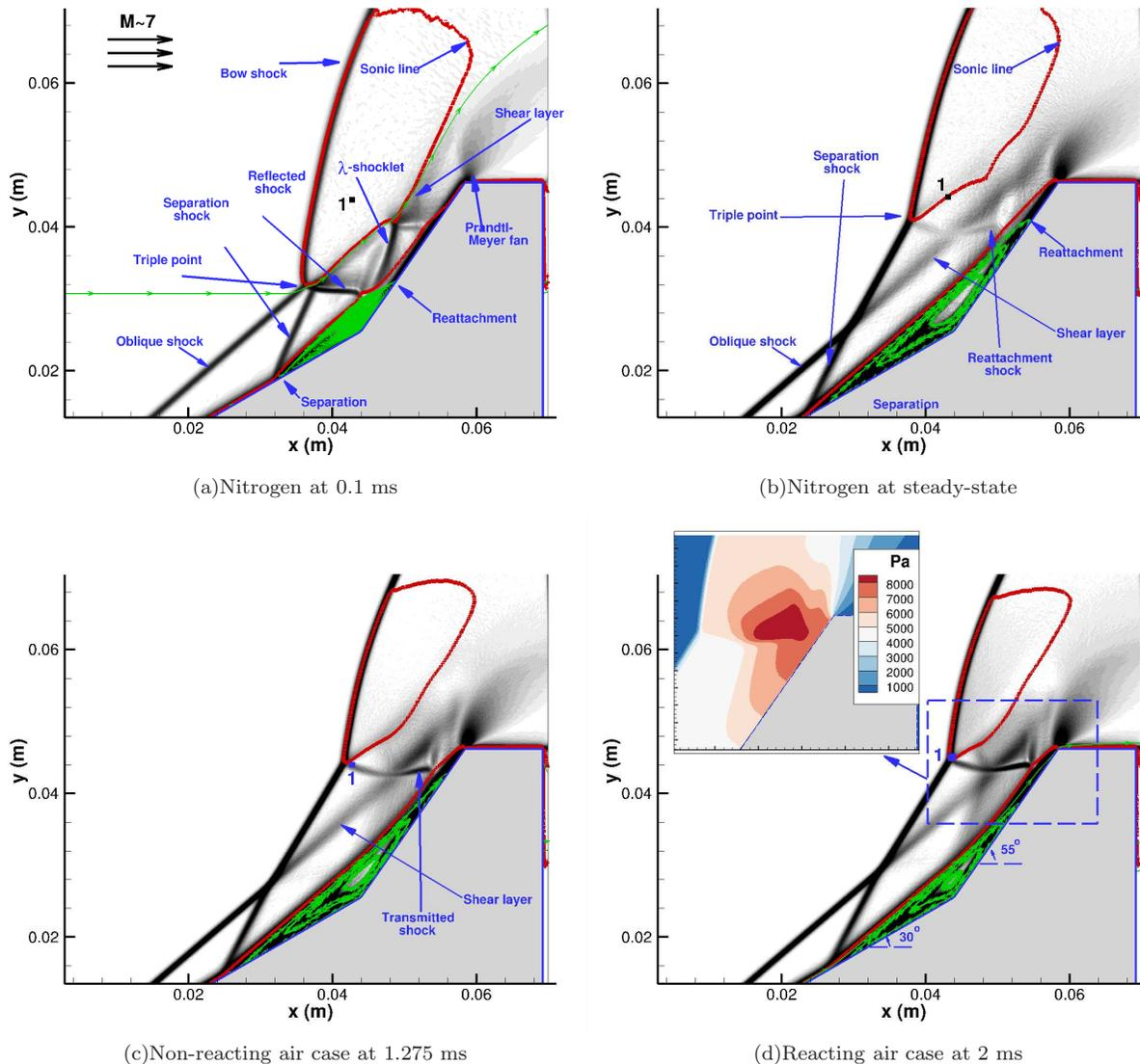
FIG. 1. Transient shock structure prior to steady state, except for Fig. 1b, for different gas species based on computed Schlieren of this work. The inset shows the spatial distribution of the pressure values in the vicinity of the second cone surface. See Sec. IVD for estimates of times to reach steady state. See also Supplemental Material in Ref. [20] for the time evolution of the flow field parameters.
