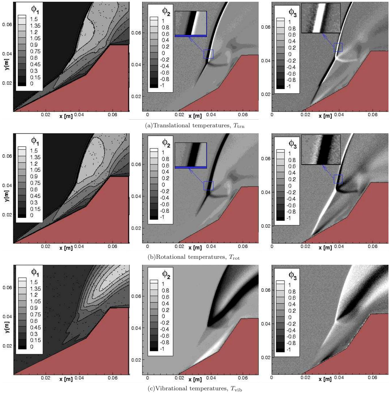
FIG. 6. Spatial distribution of POD modes for the temperature fields for the nitrogen case.
