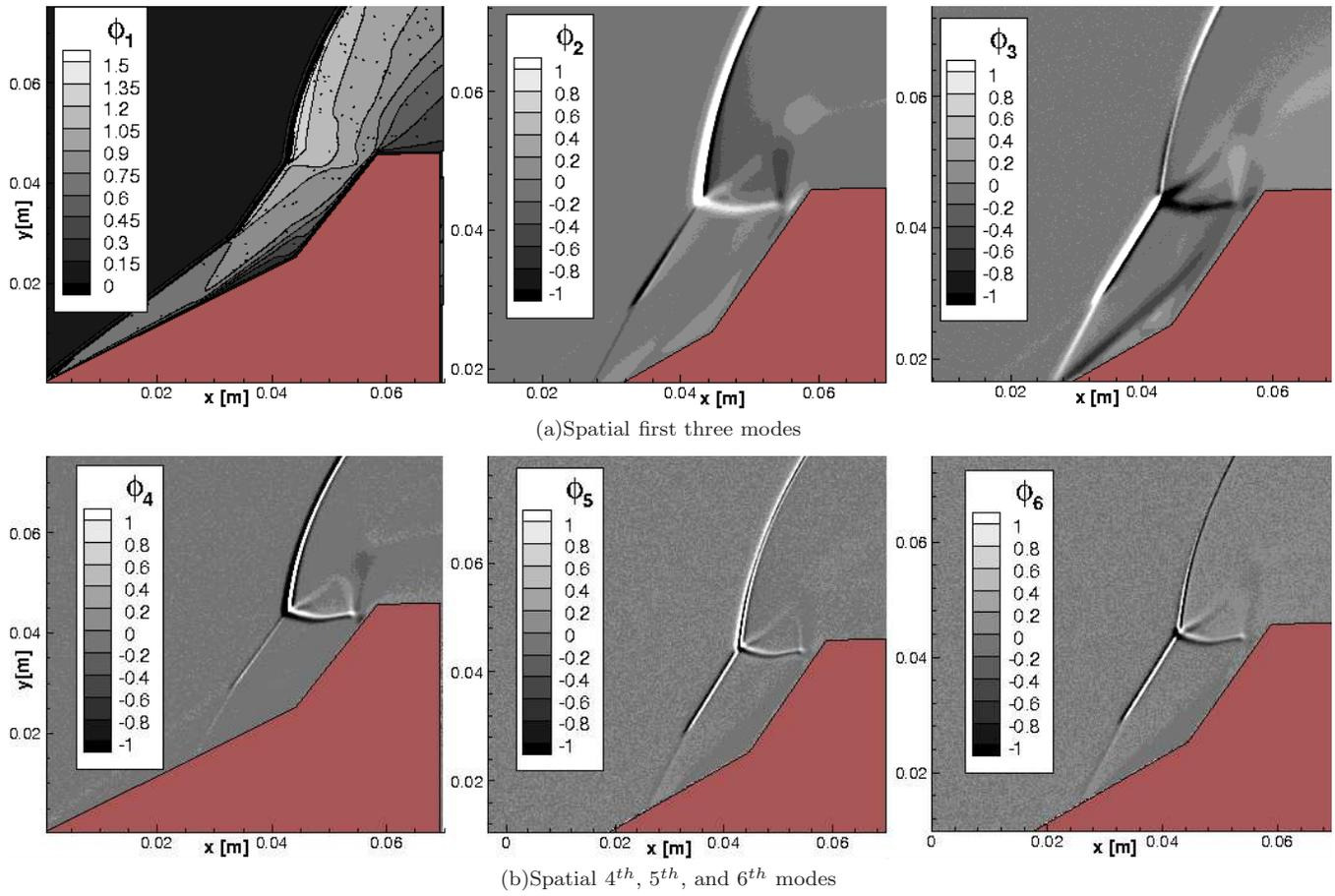
FIG. 13. POD modes for the translational temperatures of nitrogen for the reacting air case.
