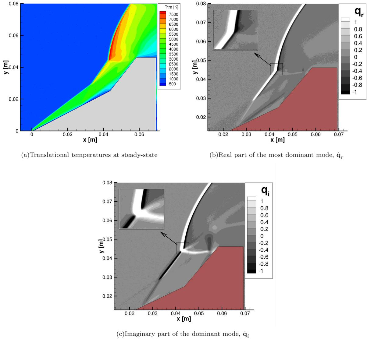
FIG. 16. Spatial distribution of the translational temperatures at steady state and amplitude functions normalized with 1000 K for the reacting air case.
