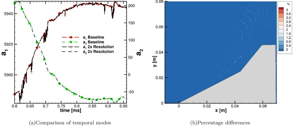
FIG. 22. Convergence of the WPOD time windows for the rotational temperatures of nitrogen molecules.
