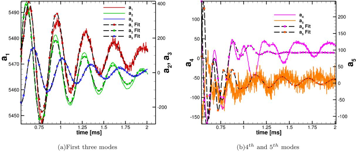
FIG. 15. Temporal modes of the translational temperature for nitrogen molecules for the reacting air case.
