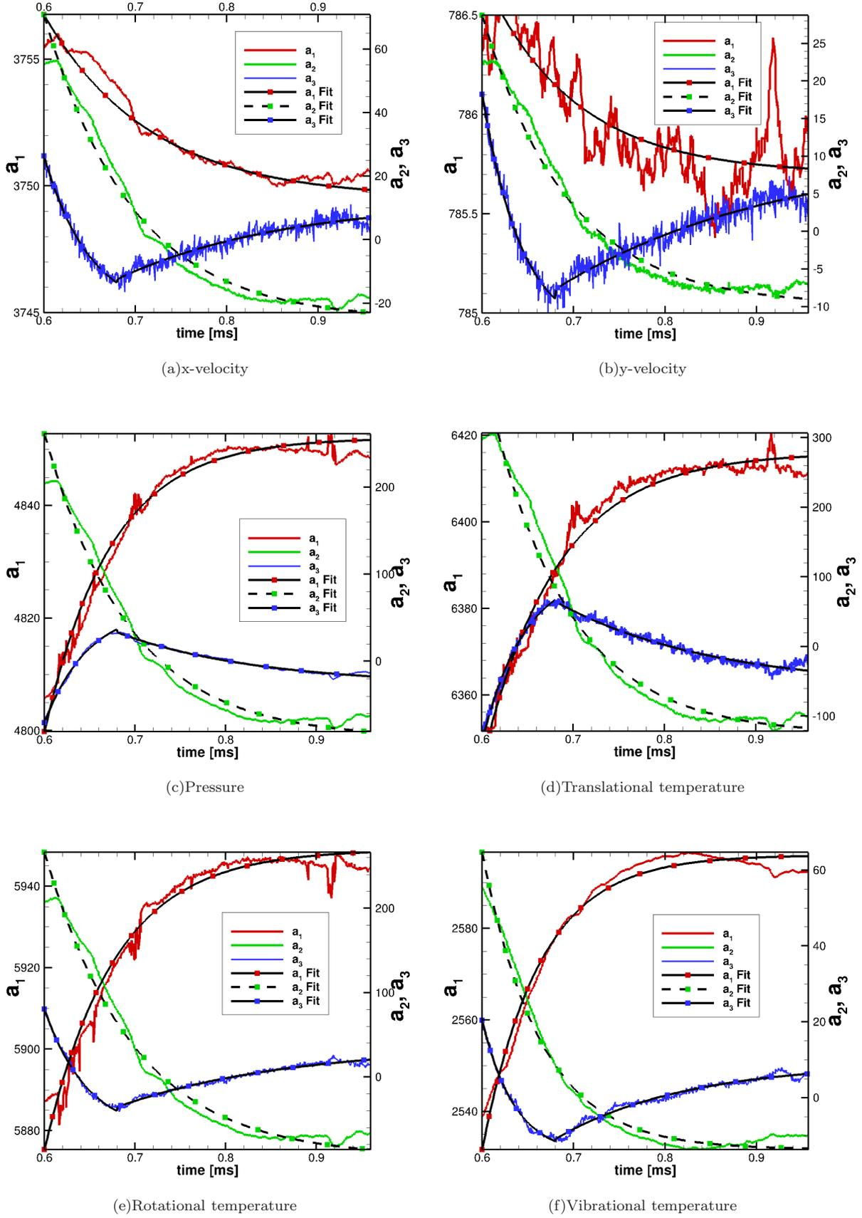
FIG. 7. Temporal parts of the POD modes for non-reacting nitrogen case.
