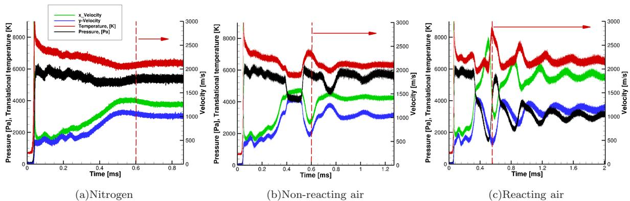
FIG. 2. Time variation of flowfield parameters in the vicinity of the triple point (see location 1 in Fig. 1). Red arrows indicate the time intervals where the WPOD algorithm will be applied.
