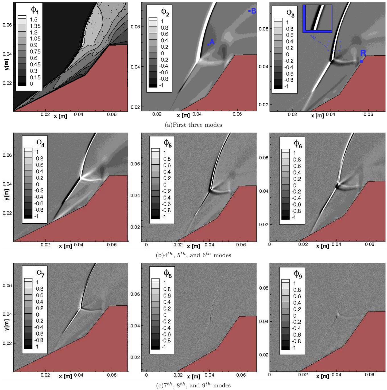
FIG. 9. Spatial parts of the POD modes for the translational temperatures for the non-reacting air case.
