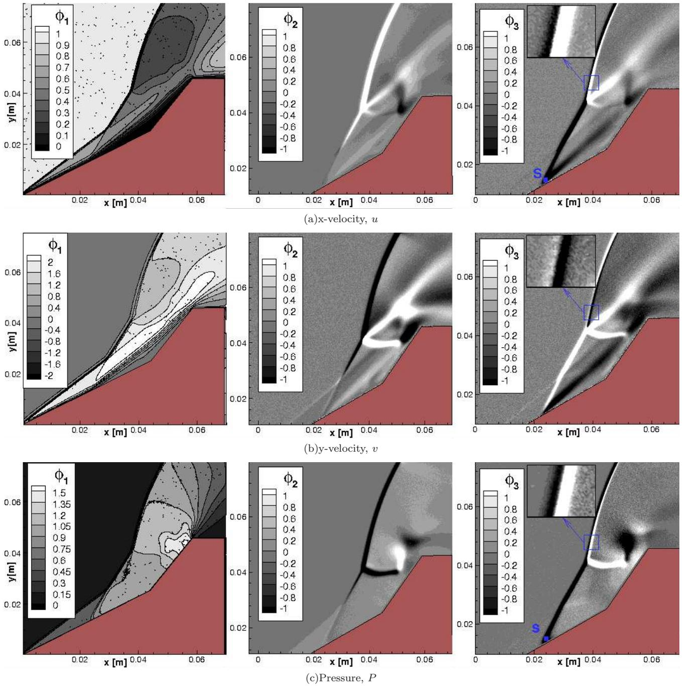
FIG. 5. Spatial distribution of POD modes for the velocity and pressure fields of nitrogen.
