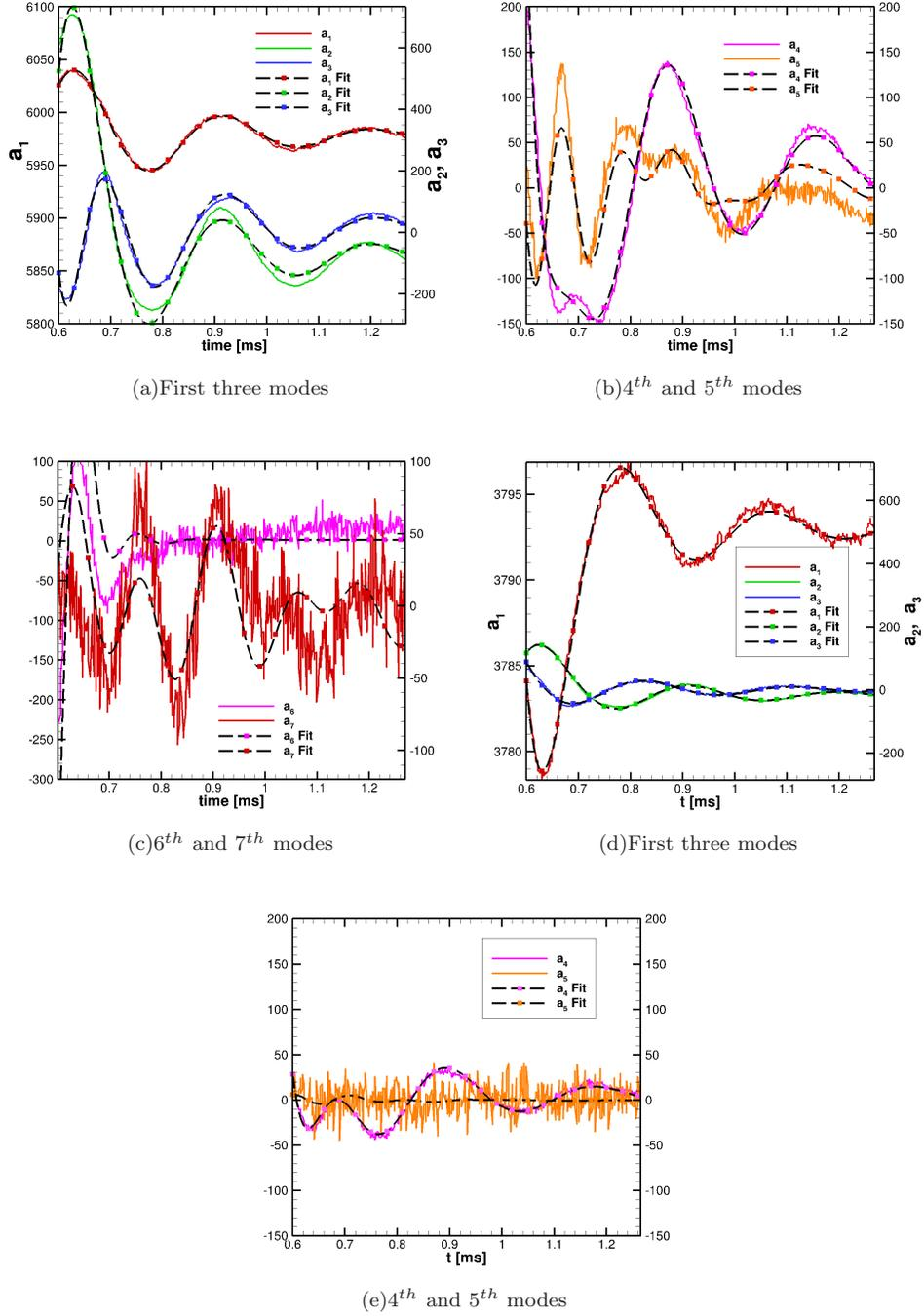
FIG. 11. Temporal parts of the modes for the non-reacting air case: (a), (b), and (c) the translational temperature for nitrogen and (d), (e) x-velocity for oxygen molecules.
