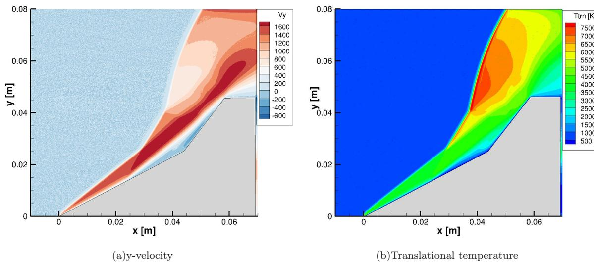
FIG. 8. WPOD predictions of steady state spatial distribution of the y-velocity and translational temperature fields for the nitrogen case.
