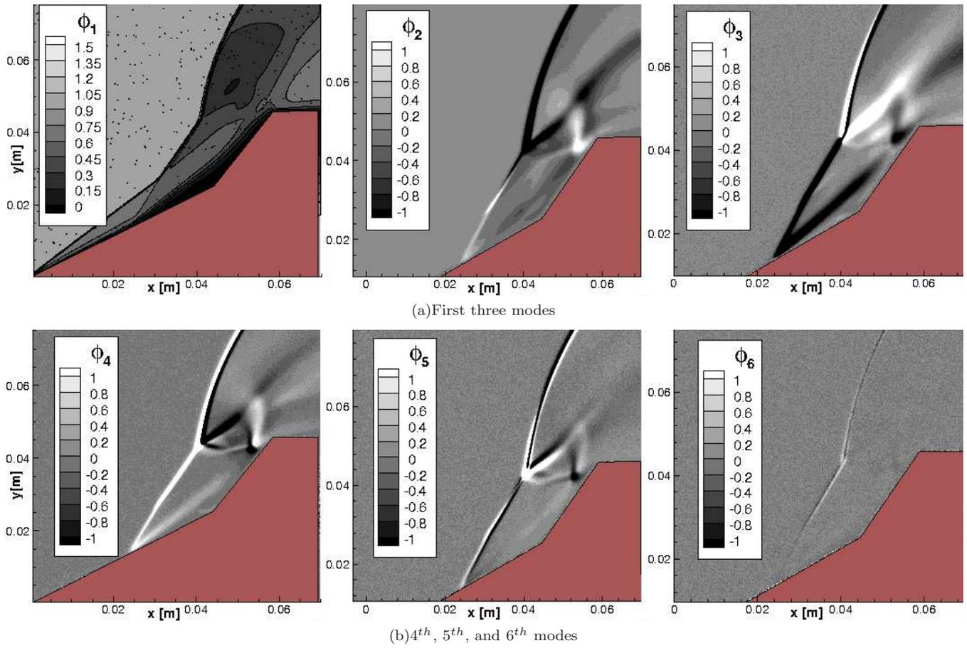
FIG. 10. Spatial parts of POD modes for the x-velocity field for the non-reacting air case.
